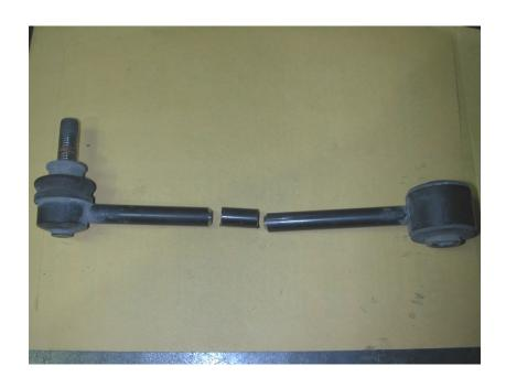
10. For necessary clearance and optimum effectiveness the sway bar end link must be shortened by approx. 1" so that it is 7 3/4" long from center eye to center eye. This 1" section will have to be cut from the center of the link and then welded back together.
