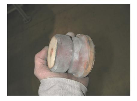
6. One of the convolutions of the bump stop must be removed to allow maximum drop. This picture shows it after cutting.
