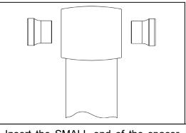
Insert the SMALL end of the spacer INTO each side of the center pivot ball. Push the spacer in until it bottoms out in the center pivot.
