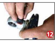
Install upper spring mount retainer clip (803-00-199) into the groove on the upper eyelet as seen in figure 12. Then, reinstall adjuster to complete assembly.
