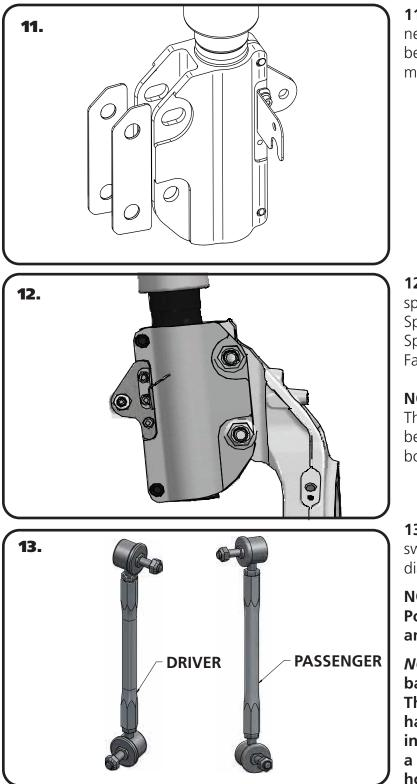
**11.** The Kit includes 4 shims. A shim will need to be placed on each side of the spindle, between the spindle and each ear of the strut mount.
