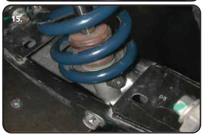
**13.** Install the shock body side of the CoilOver Assembly(1) into the upper mount(2) using a (90002403) spacer(3) installed into the bearing. With the spacers installed into the shock bearing, insert the Coilover into the mount aligning the holes in the mount with the thru hole in the bearing spacers. Install a 1/2" Flatwasher(4) on the 1/2 x 2 1/2" Hex bolt(5) and insert in the aligned holes. Finish by installing a 1/2" Flatwasher(4) and 1/2" Nylok nut(6) and torque the nut/bolt to 50 ftlbs.
