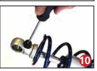
Before the upper spring mount can be installed screw the adjuster knob on the upper eye mount to the firmest setting (clockwise) as seen in figure 10. Then remove the Knob by holding it while removing the center screw.
