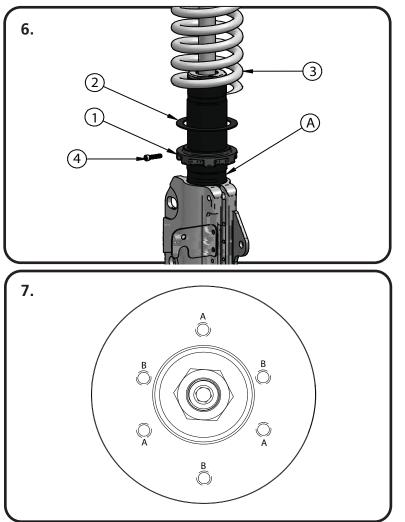
**6.** Install the Coilspring on to the Strut (A) according to Diagram #6.
