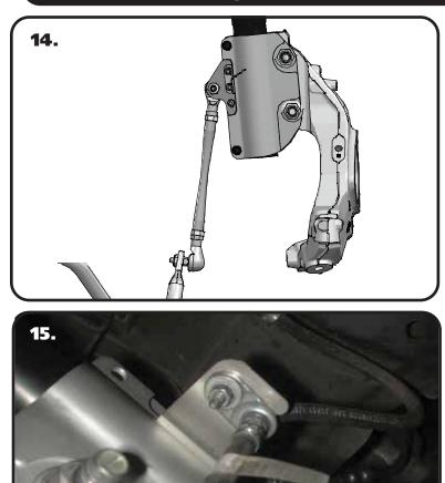
**14.** The PosiLink mounts with the stud on the Strut pointing forward, and the stud on the Sway bar pointing in.
