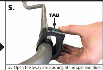
5. Open the Sway Bar Bushing at the split and slide it OVER the Delrin Liner. The Bushing needs to installed with the TAB upward and the radius to the rear. Do this on both Delrin Liners. Images 5 & 6 illustrate the correct positioning of the bushings.
