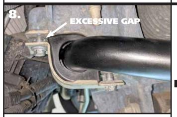
**8.** If you are experiencing an excessive gap between the cradle and bushing straps, install the (4) supplied spacers between the strap and cradle. Excessive gap would be 5/16" or more.
