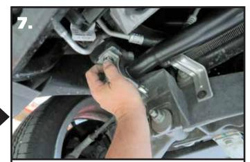
**7.** While holding the swaybar in position, reinstall the OEM bushing straps using the OEM hardware. Leave the hardware loose until the linkage is attached to the swaybar.
