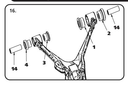
**16.** Using the Diagrams on Page 2 & 3, Insert the correct Bushings in the correct locations using a Bench Vise to push them in. Push the Bushings in followed by the correct Inner Sleeve. The Front Lower uses Bushing 1, 2, 3, 4, and Inner Sleeve 14
