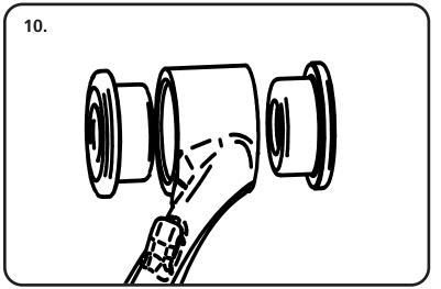
**10.** Press a set of bushings into each opening of the upper control arm. A bench vise can be used to do this.
