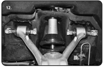
**12.** Reinstall the Control Arm on the car with any shims back into their previous location. Tighten all Fasteners.
