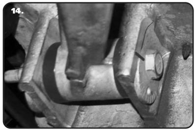
**14.** Before removing the Lower Control Arms, use a Marker or something similar to mark the Lower Control Arm Eccentrics. The marks will get the Alignment close, but Ridetech recommends getting the alignment checked after the install is completed.
