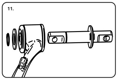
**11.** Install a Trunnion into each set of Bushings installed in the Control Arm. The Trunnions are inserted with the Shoulder to the outside of the Control Arm. Install a 3/4" Washer followed by a Snap Ring on each Trunnion.
