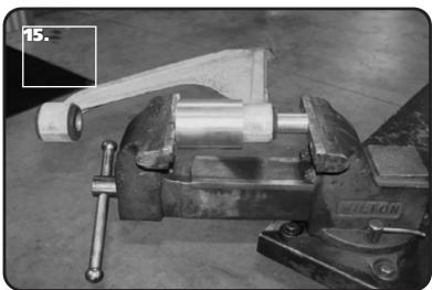
**15.** Remove the Lower Control Arm. Using the Ridetech tool (with large side over bushing) and a Bench Vise, push out the original Bushings. Clean out the opening of any debris that may have been left behind.
