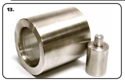
**13.** With the upper reattached, it is time to do the Lower Control Arm. Ridetech sells tool 85000006 to aid in removal of the bushings. The Tool is 2-sided with a large opening for the Lower Bushings and the opposite side being smaller for the Rear Upper Bushings. It comes with a Mandrel to insert into the center sleeve for pushing the Bushings out of the Control Arm.
