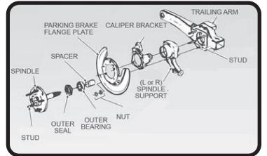
The caliper brackets are installed on the studs of the trailing arm, on top of the spindle support. The above pictures show the driver side.
