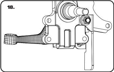
**18.** Torque the steering stop nut to 22 ftlbs.
