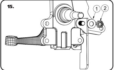
**15.** Install a 1/2" flat washer (1) and 1/2" thin nylok nut on the threads of the bolt sticking through the steering stop.
