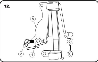
**12.** Install a 1/2" flat washer(1) on 1/2"-13 x 2" **FULLY THREADED** hex bolt(2) and insert it through the bracket(A) and spindle. This will help hold the bracket in position while tightening the 5/8" bolt. The welded on bung of the bracket should sit against the back side of the spindle. Torque the 5/8" bolt to 130 ftlbs. Torque the 1/2" bolt to 75 ftlbs.
