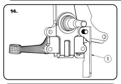
**14.** Slide the steering stop in place. The top tab goes on the wheel side of the spindle, opposite of the caliper bracket. It will slip onto the threads of the bolt that is sticking through the face of the spindle. The bottom tab is positioned over the steering arm hole.
