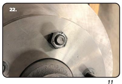
**22.** To help ease caliper installation, thread a lug nut onto a stud to hold the rotor in place.
