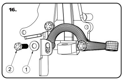
**16.** Align the steering stop and steering arm with the threaded hole of the spindle. They will be held in place with a 1/2" flat washer (1) on a 1/2"-20 x 2" hex bolt(2). Apply red loctite on the threads of the bolt.
