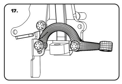
**17.** Insert the bolt/washer through the steering stop and steering arm. Thread the bolt/washer into the spindle. Torque the steering arm bolts to 100 ftlbs.
