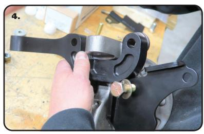
**4.** Align the Steering Arm mounting holes with the 2 bottom holes of the spindle. The steering arm will be pointing the opposite direction of the caliper bracket. Again, this is the passenger side with the steering arm going to the rear of the car.
