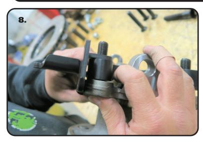
**8.** Insert a 2nd 1/2"-20 x 2 1/2" flat head socket cap screw through the spindle, steering arm, and steering stop. Install a 1/2"-20 nylok nut.
