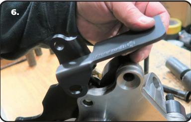
**6.** Slide the Steering Stop in place. The top tab goes on the wheel side of the spindle, opposite of the caliper bracket. The bottom tab is positioned over the steering arm hole.
