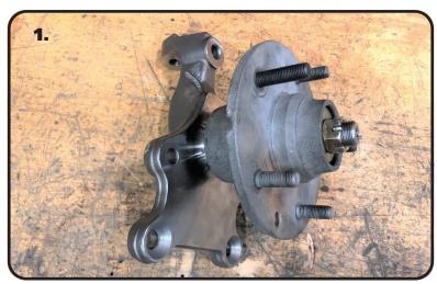
**1.** Start be greasing the wheel bearings and installing the hubs on the spindle using the nut, washer, and cotter pin supplied with the kit.
