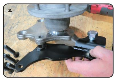
**2.** Apply Red Loctite to the 5/8"-18 x 1" bolt supplied with the spindle. Using **Image 2** as a reference, line up the 5/8" hole of the bracket with the threaded hole near the top of the spindle. Insert the 5/8" bolt through the hole in the bracket and thread it into the spindle. Pictured is the passenger assembly, it positions the caliper on the front side of the spindle
