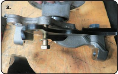
**3.** Install a 1/2" flat washer on 1/2"-13 x 2 1/4" hex bolt and insert it through the bracket and spindle. This will help hold the bracket in position while tightening the 5/8" bolt. The welded on bung of the bracket should sit against the back side of the spindle. Torque the 5/8" bolt to 130 ftlbs.
