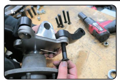
**5.** Insert (1) 1/2"-13 x 2 1/2" flat head socket cap screws through the spindle and steering arm. Install a 1/2"-20 nylok nut on the bolt closest to the end that attaches the tie rod.
