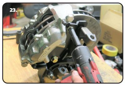
23. Install the caliper in place, making sure you have the correct caliper on the correct side. The bleeder should be to the top of the caliper. Install a 7/16" split lock washer on each of (2) 7/16"-20 x 1 1/4" bolts. Line up the threaded holes in the caliper with the mounting holes in the caliper bracket. Insert the 7/16" bolts through the caliper bracket, threading them into the caliper. Torque bolts to 70 ftlbs.
