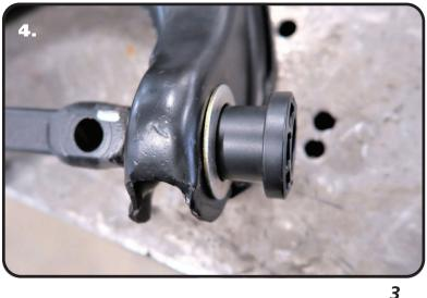
**Note:** The Delrin is self-lubricating, no lubricant is needed.
