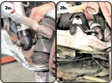
**2a.** Attach the Trunnion to the OEM control arm using the OEM hardware. It made be necessary to rotate the Trunnion to get it in the correct position. This can be done by sticking a screwdriver in one of the slots and spinning the trunnion in the shock bushing.
