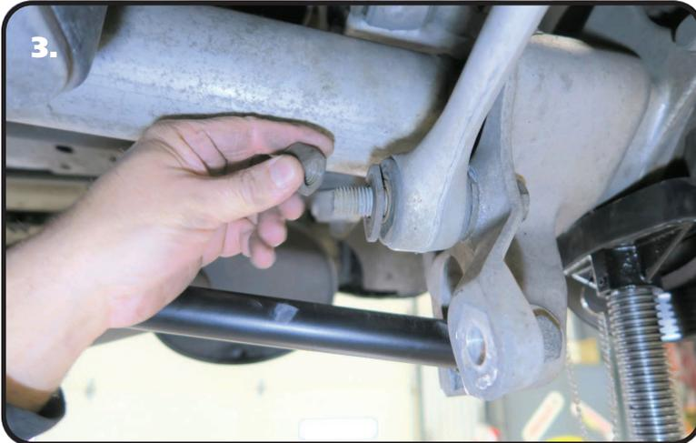
3. Remove the mounting hardware for the rear lower trailing arm. **Retain the OEM washers that are on each side of the trailing arm bushings, they will be reused during the installation of the new trailing arm.** The nut and bolt will be replaced with new ones that are included in the kit.
