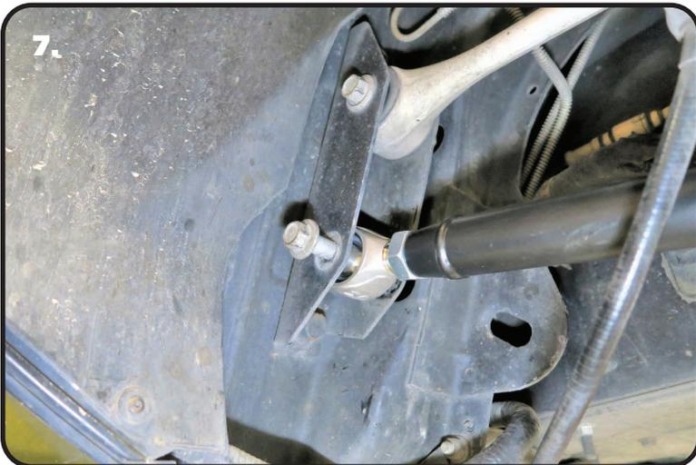
7. Line up the thru hole of the R-joint with the mounting holes in the front mount. Install a 1/2" flat washer on a 1/2"-13 x 2 3/4" hex bolt and insert in through the lined up holes. Push the bolt in far enough to get through the inner mount, but do NOT push it all the way in. You need just enough bolt sticking through to get a 1/2" flat washer on the threads.
