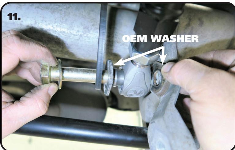
**11.** Install the second OEM washer on the threads of the bolt. At this point, you should have an OEM washer on each side of the R-Joint. Line the bolt up with the OEM mounting hole that is in the knuckle. Insert the bolt into the mounting holes of the knuckle.
