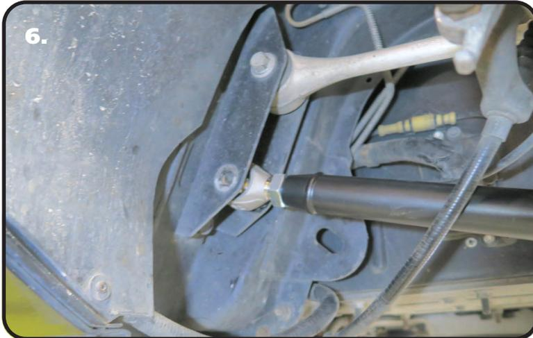
6. Insert the R-joint with the 1/2" ID spacers installed into the front mount.
