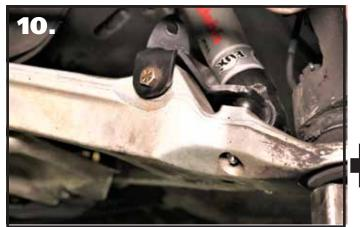
**10.** Install a 3/8"-16 x 2 3/4" bolts through the bracket and OEM linkage location. Install a 3/8" flat washer and 3/8"-16 nylok nut on the threads of the bolt that are sticking through the bracket. Do Not Tighten until the shock bolt has been installed.
