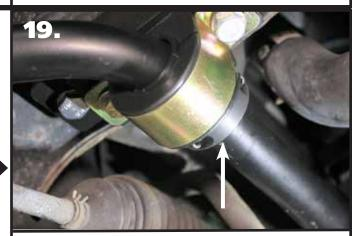
**19.** Disassemble the Locking Rings provided in the kit. The locking rings will need to be installed against the inside edge of the swaybar bushings. Assemble each locking ring against the swaybar bushing and tighten.
