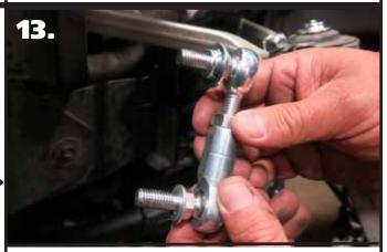
**13.** Install a T-bushing on one end of the linkage (small diameter out), with a 3/8" flat washer on the other end. The end with the T-bushing will be the TOP end of the linkage that will be installed in the swaybar end.
