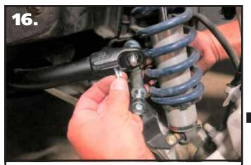
**16.** Install a 2nd T-bushing on the threads of the upper stud with the small diameter sticking into the swaybar end.
