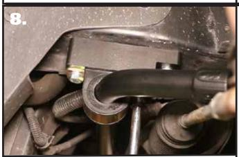
**8.** Bolt the bushing straps in place using (1) M10-1.5 x 60mm socket head caps screw and M10 flat washer in the front hole. The rear holes uses (1) 3/8"-16 x 1" bolt and M10 flat washer. Insert the hardware through the bushing strap bolting the strap in place. DO NOT TIGHTEN THE HARDWARE at this time.
