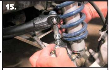
**15.** Install a 3/8" flat washer followed by a M10-1.5 serrated lock nut on the threads of the lower stud of the linkage.
