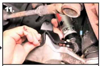
**11.** Install a 5/16"-18 x 2 1/4" bolt through the outer tab and through the shock t-bar/control arm. Install a 5/16" flat washer and 5/16"-18 nylok nut on the threads sticking through the control arm. Torgue all hardware.
