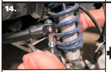
**14.** Install the Linkage with the Studs pointing to the wheel. The linkage will be installed with the previously installed t-bushing in the swaybar end.
