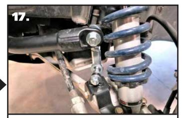
**17.** Install a M10-1.5 serrated lock nut on the threads of the upper stud of the linkage. Repeat Steps 13-17 on the other side. Torque the hardware.
