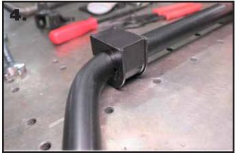
**4.** Open the Sway Bar Bushing at the split and slide it **OVER** the sway bar. Do this for both bushings.
