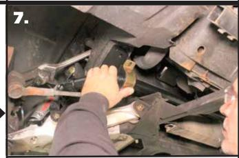
7. Install the Bushing Straps on the swaybar bushings.
