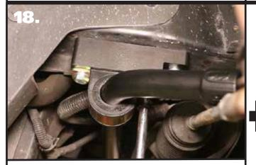
**18.** Center the swaybar on the mounts and torque the bushing strap hardware.
