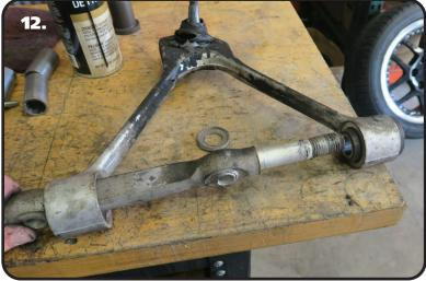
**12.** Insert the cross shaft through the side of the control arm that doesn't have a bushing installed.
