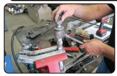
**14.** Reinstall the OEM outer washers and nuts. Torque the nuts 35-40 ftlbs.
