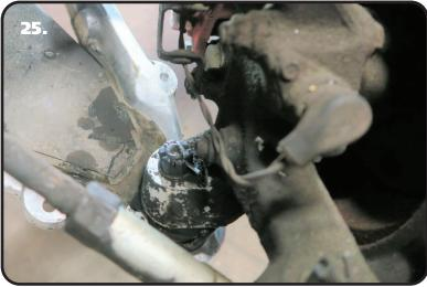
**25.** Insert the lower ball joint into the spindle. Reinstall the castle nut and torque to 50 ftlbs. Check alignment of the cotter pin hole. If it does not line up with an opening in the castle nut, tighten the nut until it does line up. Reinstall the cotter pin and bend the ends to keep it in place.
