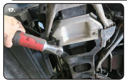
**17.** The spring travel limiter will need to be removed. There are 2 vertical bolts and 2 horizontal bolts.
