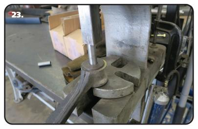
**23.** Push the inner sleeves into the Delrin bushings. We used an Arbor Press, but a bench vise will work for this.
