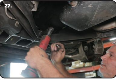
**27.** Reinstall the crossmember brace if working on a later model Corvette.
