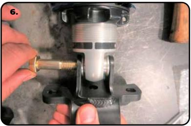
**6.** Insert the shock into the Lower Mount. Line up the shock bearing/spacers hole with the mounting holes of the lower mount. Insert a 1/2"-13 x 2 3/4" bolt through the mount/ shock. Install a 1/2" flat washer and 1/2"-13 nylok nut on the threads of the bolt that are sticking through the mount.
