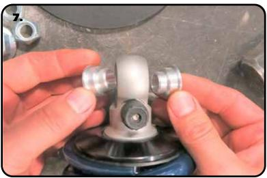
**7.** Install the 1/2" I.D. bearing spacers into bearing in the shock eyelet. These spacers have a through hole that is 1/2" diameter. The small diameter of the spacers will insert into the shock bearing.
