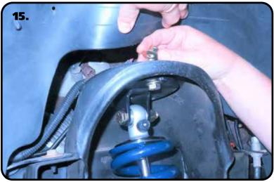
**15.** Install a 7/16" flat washer on each of (3) 7/16" -14 x 1 3/4" hex bolts. Align the mounting holes of the upper mount with the mounting holes in the frame. The mounting bolts need to be installed with the threads pointing up. Insert a bolt/washer in each holes. Install a 7/16" flat washer and 7/16"-14 nylok nut on the threads of each bolt sticking through the frame. Torque the hardware to 50 ftlbs.
