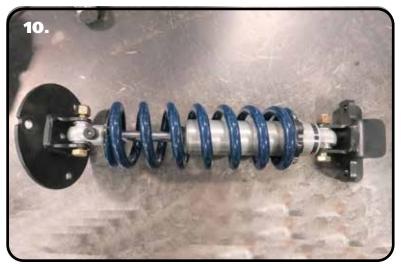
**10.** Your assembly should look like **Image 10**. The SHORT TAB of the lower mount should be on the same side as the NOTCH in the upper mount. If it is NOT, you can turn the upper mount by hand.
