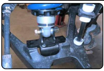
**11.** Put the CoilOver in position on the truck. The Lower Mount will only attach to the control arm one way. The SMALL vertical tab needs to be positioned toward the wheel.
