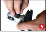
Install the locking screw in the adjuster nut before setting spring preload, but DO NOT tighten until the spring preload has been set.
