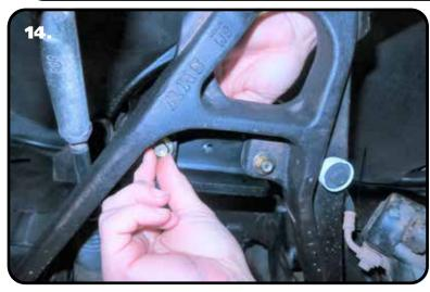
**14.** Install a 3/8" flat washer and 3/8"-16 nylok nut on the threads of the bolts sticking through the lower control arm. Torque the hardware to 45 ftlbs.
