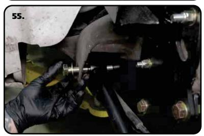
**55.** Line the through hole of the R-Joint with the holes of the leaf spring mount. Install a 5/8" flat washer on to a 5/8"-18 x 4.5" hex bolt, insert into the lined up holes. Install a 5/8" flat washer followed by a 5/8"-18 THIN nylok nut. Repeat on both sides and tighten the bolts/nuts enough to eliminate any gaps.
