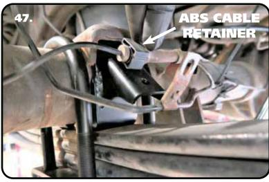
**47.** Remove the ABS cable from the retainer that is attached to the same bracket as the brake line retainer. Remove the ABS cable retainer from the bracket. These will be reinstalled later.
