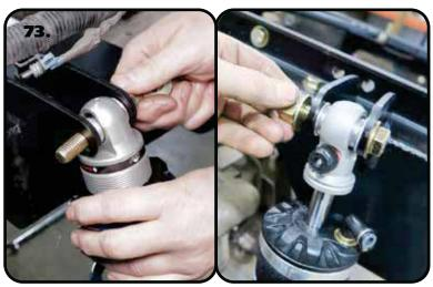
**73.** Insert the Shock with the 1/2" ID Spacers into the shock mount. Install a 1/2" flat washer on a  $1/2"-2- x \ 2 \ 1/2"$  hex bolt. Line up the holes in the mount with the spacers and shock bearing. Insert the bolt/washer into the lined up holes. Install a 1/2" flat washer & 1/2"-20 Nylok Nut. Torque to 75 ftlbs
