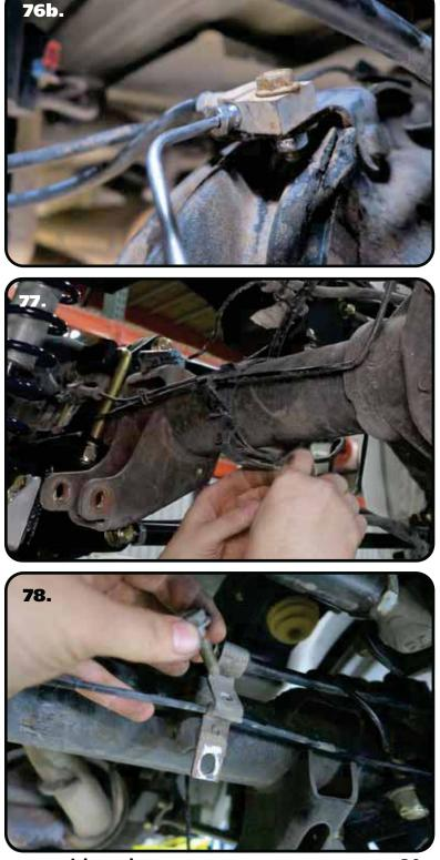
**76b.** This is the other brake line possibility. Remove the OEM brake line bracket that attaches to the differential cover bolt and brake line mount. Attach the new brake line bracket to the differential using the supplied M8-1.25 x 20mm bolt and 5/16" flat washer. Attach the brake line mount to the new brake line tab using (1)  $5/16"-18 \times 1"$  bolt, (1) 5/16"-18 nylok nut, and (2) 5/16" flat washers. Torque the M8 to 225 inlbs and the 5/16" to 17 ftlbs.
