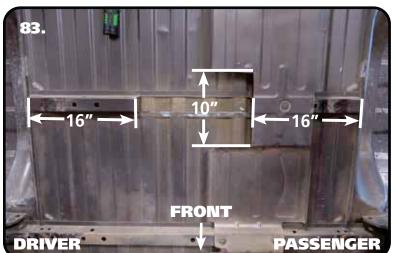
**83.** The bed brace cut starts 16" from each end of the bed brace. The heat shield on the passenger side will need notched for axle clearance. It is notched 5" forward and back from the center of the bed brace. Cut the bed brace even with the bent flange that attaches it to the bed floor.
