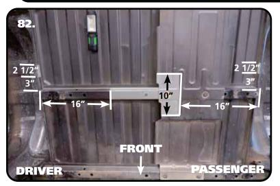
**82.** Trimming of the bed brace that is in between the wheel wells is necessary to clear the c-notches. The inside fender well lip will need to be cut to clear the shock mount. We cut ours with a die-grinder. **Image 82** shows the areas that will need cut out. **Step 83** covers the notching of the heat shield and bed brace. **Step 84** covers the cutting of the fender well lip.
