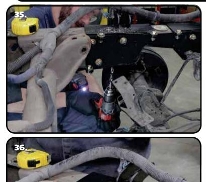
**35.** Use the c-notch as a temple to drill the hole in the bottom of the frame rail that is below the one drilled in **Step 34**. Again, use a 7/16" drill bit.
