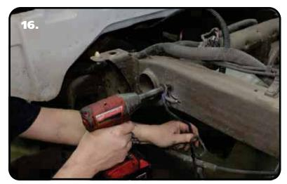
**16.** Unbolt the rear emergency brake cable bracket from the driver frame rail. Retain the hardware for later reinstallation.
