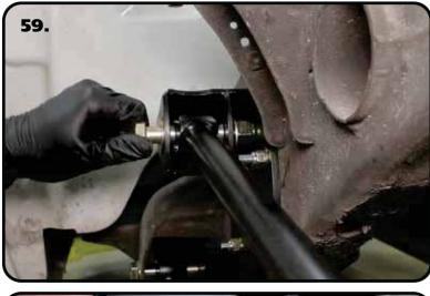
**59.** Line the through hole of the R-Joint with the holes of the bar mount. Install a 5/8" flat washer on to a 5/8"-18 x 3 1/4" Hex bolt, insert into the lined up holes. Install a 5/8" flat washer followed by a 5/8"-18 THIN nylok nut. Repeat on both sides and tighten the bolts/ nuts enough to eliminate any gaps.
