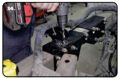
**34.** The c-notches require one hole to be drilled through the top and bottom of the frame rail. This hole is located behind the shock mount. Use the c-notch as a template to drill the hole in the top of the frame rail using a 7/16" drill bit.
