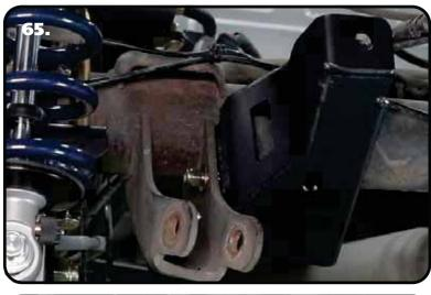
**65.** Install a 3/8" flat washer on each of (2) 3/8"-16 x 1 1/2" hex bolts. Hold the panhard mount in position and insert the bolt/washers through the mount and drilled holes. Install a 3/8" flat washer & 3/8"-16 nylok nut on each of the bolts. Do not tighten the hardware at this time.
