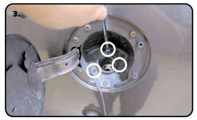
**3.** The bed will need to be removed to install this kit. Start by removing the (3) screws around the filler neck. The 3 screws are circled in **Image 3**.
