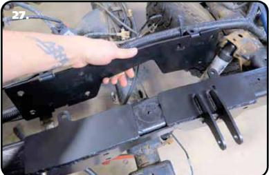
**26.** The c-notch will have a snug fit on the frame rail and will most likely need tapped in place with a dead blow hammer.
