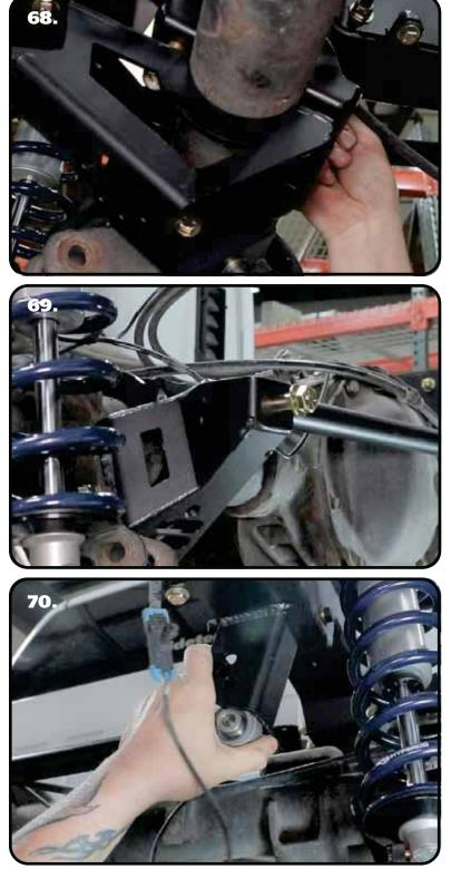
**68.** Install a 1/2" SAE flat washer on each of (2) 1/2"-13 x 1 3/4" bolts. Insert the bolt/washers in the top and bottom mounting holes of the clamp/mount. Install a 1/2" SAE flat washer and 1/2"-13 nylok nut on the threads of each bolt. Torque these bolts to 75 ftlbs. You can now torque the 3/8" hardware that was installed previously. Torque the 3/8" hardware to 45 ftlbs.
