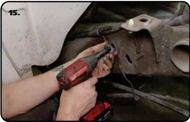
**14.** Unbolt the brake line bracket from the top of the driver frame rail.
