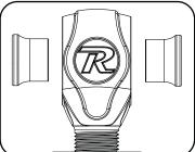
New R-Joints will be quite stiff (75-90 in/lbs breakaway torque) until they "break in" after a few miles of use. After the break in period they will move much more freely. Because the composite bearing race contains self lubricating ingredients, no additional lubrication is needed or desired. Any additional lubrication will only serve to attract more dirt and debris to the R-Joint and actually shorten its life.
