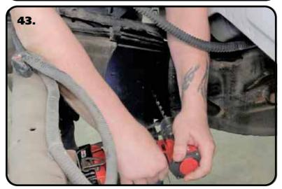
**43.** Drill the (3) inner holes that are BLACKED OUT in **Image 37** using a 3/8" drill bit. Use the inner retainer as a template.
