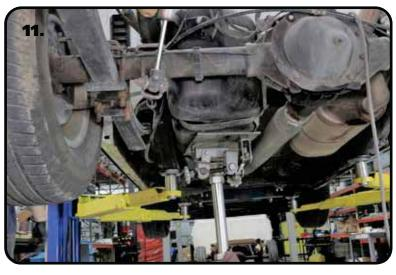
removing the gas tank straps. We use a transmission jack to support it. Remove the gas tank strap hardware and straps. Slowly lower the gas tank.
