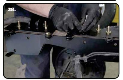
**28.** Install a 3/8" flat washer on each of (6)  $3/8"-16 \times 11/4"$  hex bolts. Insert a bolt/washer in each of the bolt tabs.
