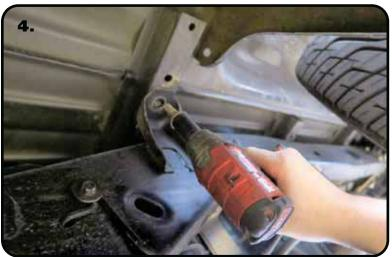
**4.** Remove the hardware that attaches the bed to the frame. Unplug the tail light wiring from the rear distribution block. We suggest recruiting a few friends to lift the bed off the truck. You will want to position the bed in a way that you have access to the bottom of the bed for later modifications.
