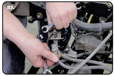
**85.** The brake line bracket that bolted to the top of the driver frame rail will need to be replaced with one supplied in the kit. Start by loosening the lines using line wrenches.
