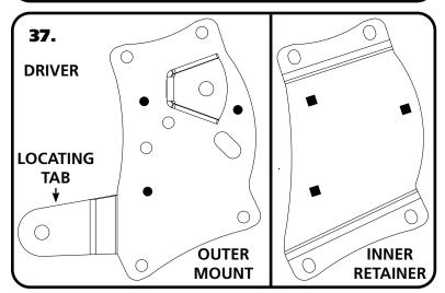
**37.** The upper bar mount consists of an outer mount and inner retainer. The outer mount has a forward locating tab that is located off the OEM front leaf spring mount. The inner retainer will wrap round the top and bottom of the frame rail. The frame rail will need to be drilled in the areas that are **SOLID BLACK** in **Image 37** after the mount is installed.
