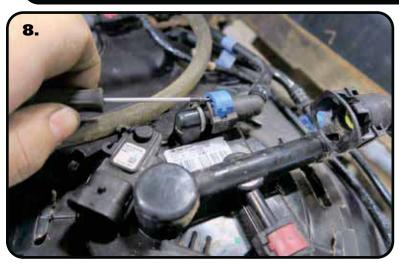
**8.** Some of the lines have a lock. It will need to be disengaged to remove the lines.
