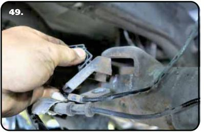
**49. Image 49** illustrates the bracket cut off. Again, we use a saw-z-all to cut it off.
