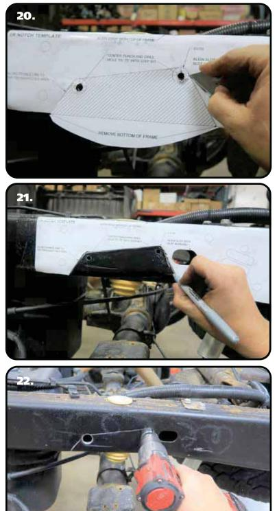
**20.** Use a razor blade to cut out the hashed area of the template.
