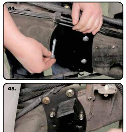
**44.** Install the (3) 3/8"-16 x 4" carriage bolts from the **INSIDE** of the frame with the threads sticking through the outer mount. Make sure the square shoulders of the carriage bolts are engaged into the square openings of the inner retainer.
