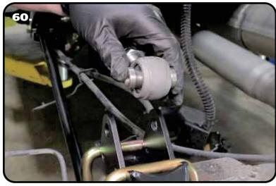
**61.** Line the through hole of the R-Joint with the holes of the axle bracket. Install a 5/8" flat washer on to a 5/8"-18 x 3 1/4" hex bolt, insert into the lined up holes. Install a 5/8" flat washer followed by a 5/8"-18 THIN nylok nut. Repeat on both sides and tighten the bolts/ nuts enough to eliminate any gaps.
