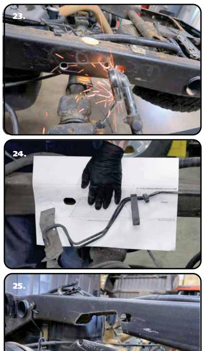
**23.** Remove the template and cut the line you just traced.
