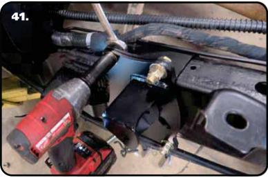
**41.** Install a 1/2" flat washer on each of (4) 1/2"-13 x 1 1/2" hex bolts. Insert the bolt/ washer through the (2) top holes & (2) bottom holes of the outer mount and inner retainer. Install a 1/2" flat washer & 1/2"-13 nylok nut on each of the (4) bolts. Torque to 80 ftlbs.
