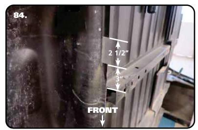
**84.** The inside fender well lip needs to be cut to clear the shock mount. The rear of the cut out is 3" behind the bed brace. The cut out needs to be 2 1/2" long.
