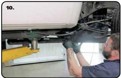
**10.** Remove the gas tank shield hardware and remove the gas tank shield.
