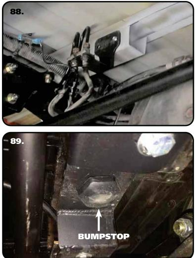
**88.** Slip the brake line(s) into the new bracket and reinstall the clips. Screw the brake line bracket to the bed brace using the supplied #10 x 3/4" self drilling screws.
