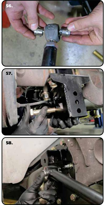
**56.** Insert (2) .625" ID x .740" long R-Joint spacers into the R-Joint of one end of each lower bar. The small diameter of the spacer goes into the R-Joint. Insert the rear of the lower bar R-Joint into the lower axle bracket.
