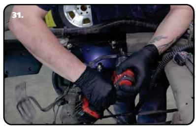
**29.** Install a 3/8" flat washer and 3/8"-16 nylok nut on each of the (6) bolts. Torque to 45 ftlbs.
