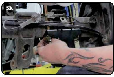
**53.** Hold the mount in place and install a 5/8" flat washer and 5/8" high nut on the threads of the u-bolts sticking through the axle mount. Tighten the nuts evenly in a criss-cross fashion making sure the tabs of the axle mount are touching the leaf spring pad evenly. Torque the nuts in a criss-cross fashion to 60 ftlbs. Repeat on the other side.
