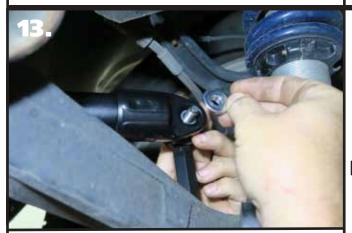
**13.** Install a 2nd t-bushing with the small diameter into the swaybar.
