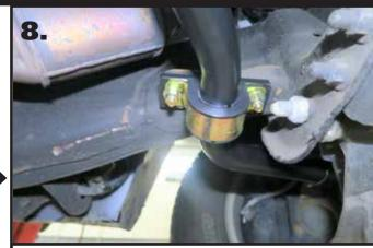
**8.** Install a 3/8" flat washer and 3/8"-16 nylok nut on each of the 4 studs. Roughly center the bar and torque the nylok nuts.
