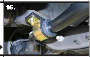
**16.** Install the stop rings against the swaybar bushing. The stop rings will go against the inner side of the bushing. Take the stop rings apart and reassemble them against the bushing and tighten.
