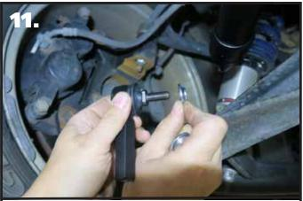
**11.** Install a T-Bushing on each of the 90 degree end links. The t-bushings are installed with the large diameter against the shoulder of the end link.
