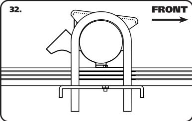
**32.** Slip the Leaf Spring Bracket up onto the U-Bolts WITH THE OFFSET HOLE FORWARD. THE ARROW ON THE BRACKET SHOULD POINT TO THE FRONT OF THE TRUCK.
