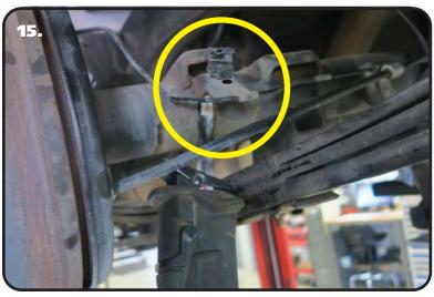
**15.** The bracket that is at the rear of the OEM leaf spring perch will need to be cut off of the axle tube. We use a saw-z-all to cut it off. It needs to be cut off even with the axle, perpendicular to the top of the leaf spring perch. Use **Images 15 & 16** as a reference.
