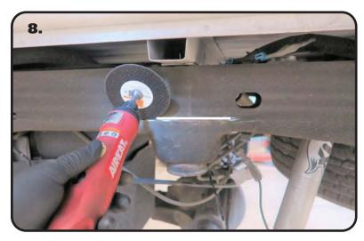
**8.** The OEM bump stop mount will need to be cut off the frame. We do this by cutting the weld with a cut off wheel on a die-grinder. Cut in the center of the weld without going too deep. Cutting too deep will cut into the frame.
