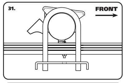
**31.** Slip the U-Bolts over the axle tube with the threads pointing down.
