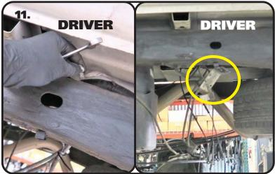
**11.** Unbolt the brake line bracket from the top of the drivers side frame rail. This will help provide enough slack in the lines to be able to flip the leaf springs on the bottom side of the axle. Retain the hardware, this bracket will be reinstalled later.
