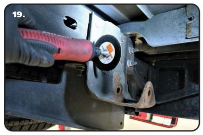
**19.** The rear leaf spring hanger will need to be removed from the frame. It is held on by (1) bolt and (3) rivets. Remove the bolt and retain it for installation of the new hanger. We remove the rivets by cutting a " + " in the rivet head and chiseling if off. After chiseling the head off, drive the rivet out of the hanger/ frame with a punch.
