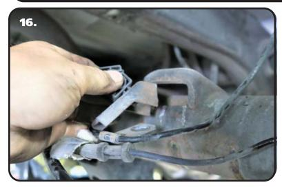
**16. Image 16** illustrates the bracket cut off. Again, we use a saw-z-all to cut it off.
