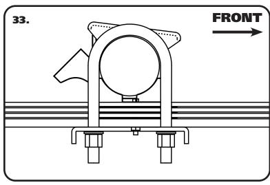
**33.** Hold the Leaf Spring Bracket in place and install a 5/8" Flat Washer & 5/8"-18 High Nut on the threads of the u-bolts. Snug the nuts down evenly and tighten them in a criss-cross fashion to 130 ftlbs.
