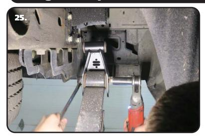
**25.** Install the shackle on the rear eyelet of the leaf spring with the open side facing the front of the truck. Align the mounting hole with the leaf spring bushing. Install the OEM hardware that was removed earlier. Repeat on the second spring. Do not tighten the hardware at this time.
