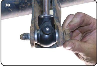
**38.** Attach the EYELET of the Shock in the OEM mount that is on the axle housing. Attach the shock using the OEM hardware. Position the Shock with the Adjuster Knob pointing out, away from the axle.
