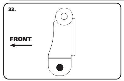
**22.** The rear shackle will get mounted in the hanger with the open side facing the front of the truck.
