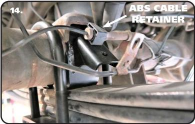
**14.** Remove the ABS cable from the retainer that is attached to the same bracket as the brake line retainer. Remove the ABS cable retainer from the bracket. These will be reinstalled later.
