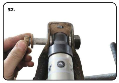
**37.** Install the BODY of the shock in the OEM frame mount using the OEM hardware.
