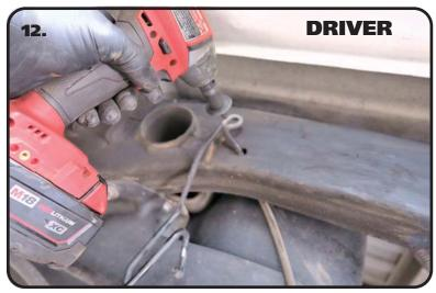
**12.** Remove the emergency brake cable holder from the driver side frame rail. Again, this bracket will be reinstalled later.
