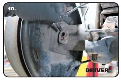
**10.** Remove the ABS sensors from the axle tubes on driver and passenger side. DRIVER SIDE IS SHOWN IN **IMAGE 10**.
