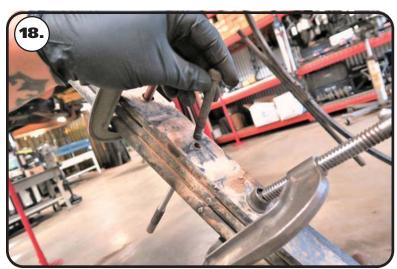
**18.** Remove the locating pin from the leaf spring pack. Reinstall the locating pin from the TOP side. Reinstall the nut on the BOTTOM side and tighten. With the nut tight, remove the clamps. Repeat on the second spring.
