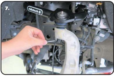
**7.** Install the ball joint nut on the ball joint pin.
