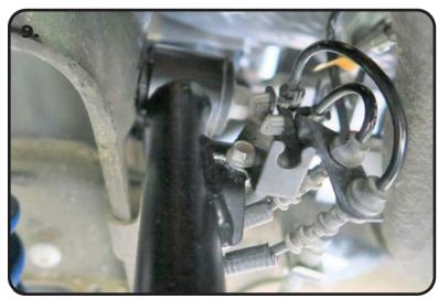
**9.** Attach the brake line bracket to the tab of the upper control arm using the OEM hardware. Torque to 92 in-lbs.
