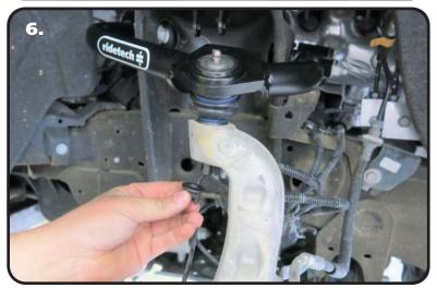
**4.** The upper control arm is attached in the factory mount using factory hardware. The driver side arm is shown in **Figure "3, 4 & 5"**. Line up the through holes of the bushings with the OEM holes.
