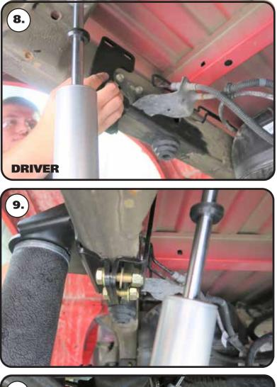
**8.** Hold the inner plate in position. It is bent to wrap under the frame rail. The (4) bolt holes will line up with the bolt holes of the upper air spring mount.
