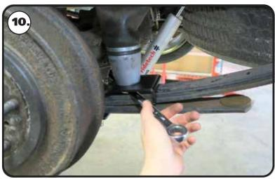
**10.** Tighten the lower 3/8" air spring bolt using a 9/16" wrench.
