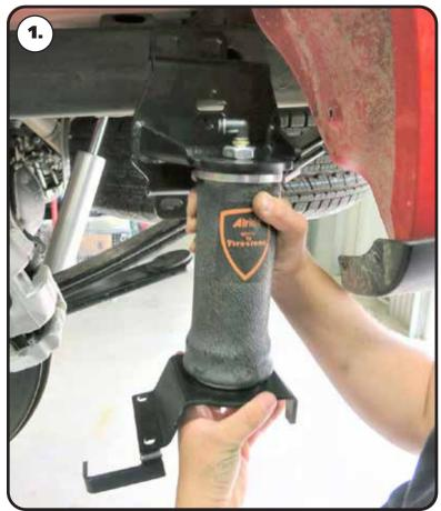
The air springs and brackets need to be assembled. The upper air spring mounts are the same for driver and passenger. The lower air spring brackets are side specific. See Image
