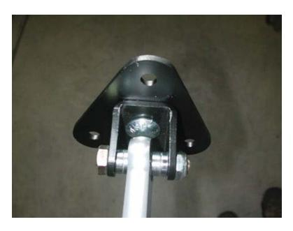
8. Insert a ½" ID shock bearing spacer in each side of the shock bearing. The small OD will go into the bearing. Bolt the Shockwave to the eye to stud adapter using the ½" x 2 ¼" bolt and Nylok nut.
