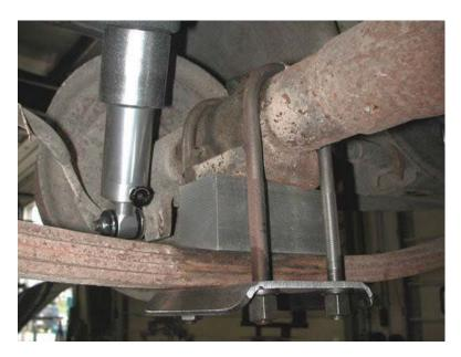
7. Hang the U-bolts over the axle. Position the U-bolt plate under the leaf springs so that the smaller hole in the plate aligns with the Allen bolt and nut. Secure the assembly with the four 5/8" nuts and lock washers supplied.
