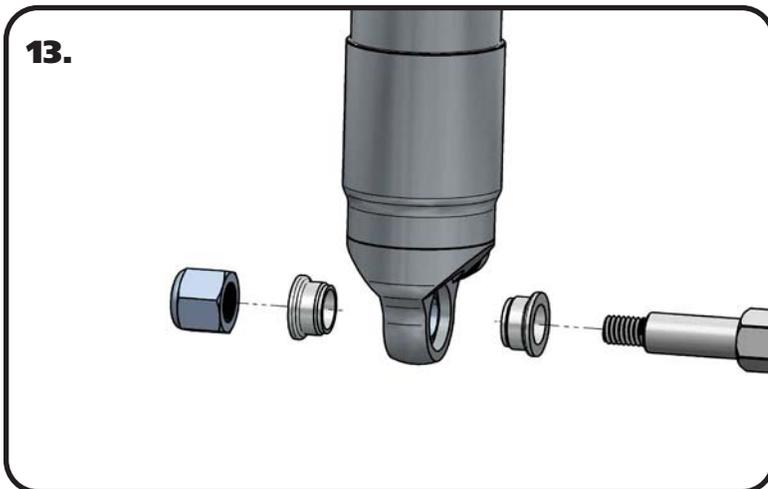
**13.** Install a 5/8" ID spacer( Small side towards shock body) onto the lower Shock Stud. Slide the bottom of the Shock onto the Stud. Install a second 5/8" ID Spacer onto the Stud(small side towards shock). You may need to jack the rearend up to Slide the Shock onto the Stud. Install the 7/16" Flat washer and 7/16" Nylok nut. Tighten the upper and lower shock bolts.
