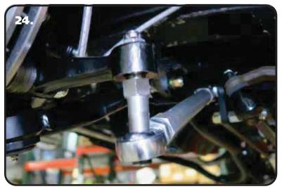
**24.** Install the outer end of the tie rod on the steering arm stud.
