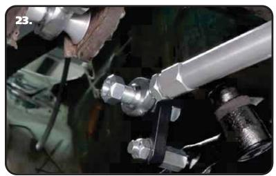
**23.** Install one end of the tie rod onto the stud of the centerlink adapter. Install a 5/8"-18 mechanical locking nut on the threads of the stud and torque to 45 ftlbs.
