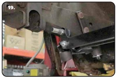
**19.** Install the 5/8"-18 **THIN** mechanical locking nut on the threads of the stud sticking through the centerlink adapter and torque to 45 ftlbs.
