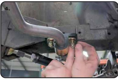
**4.** Slide the sway bar into position on the car. The sway bar arms will be bending upward with the center dropping toward the ground. Install a 3/8" x 5/8" OD flat washer on (4) 3/8"-16 x 1 1/4" socket head bolts. A bolt/washer will go in each of the 4 mounting holes. With the bolt/washers installed, install a 3/8" flat washer on the threads followed by a 3/8"-16 nylok nut. Do **NOT** completely tighten the hardware. It will be left partially loose until the end links are installed.
