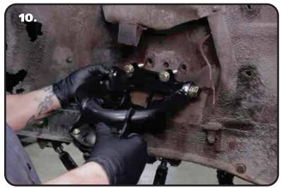
**Note:** The upper arm mounting holes on many cars have been redrilled 1" lower. This is done to improve the handling. Our cross shaft has the drop built into it; **make sure to use the factory mounting holes.**
