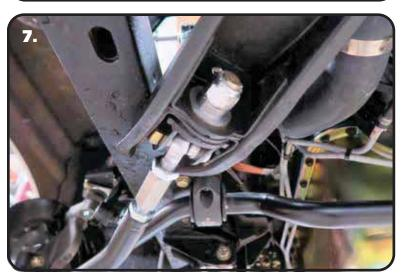
**7.** Install a 3/4"-16 nylok nut on the threads of the bolt sticking through the t-bushing. Torque to 120 ftlbs.
