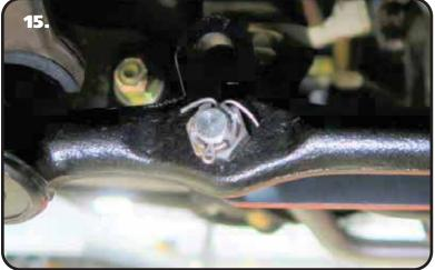
**15.** Torque the nuts to 35 ftlbs and tighten as needed to align cotter pin. Install cotter pin and bend the ends.
