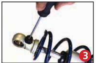
Before the upper spring mount can be installed screw the adjuster knob on the upper eye mount to the firmest setting (clockwise) as seen in figure 3. Then remove the Knob by holding it while removing the center screw.
