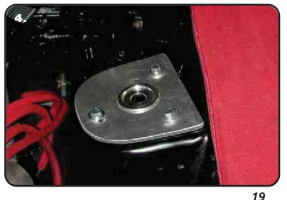
**4.** Lay the Upper Plate on Top of the shock tower with the ShockWave Mount protruding through the large center hole. Line up the the holes in the Upper Plate with the holes drilled in the shock tower and the holes in the ShockWave mount. If the INNER Hole doe not line up, flip the plate over. Install a 5/16" x 1" Flange Bolt in each hole and tighten.
