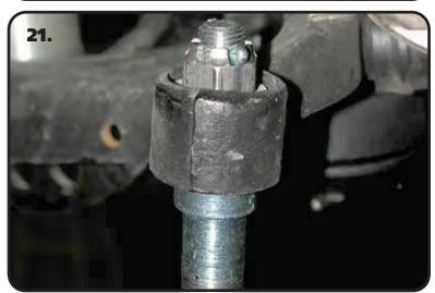
**21.** Install the stud with the round flange into the steering arm with the taper going into the steering arm. Torque the nuts to 35 ftlbs and tighten as needed to align cotter pin hole and install cotter pin.
