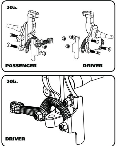
**20a.** Install the steering arms and steering stops onto the spindle using **Images 20a & 20b** as a reference. The steering arms angle toward the centerlink, and the tie rod mounting holes are to the rear of the car. The steering stops are marked D and P.
