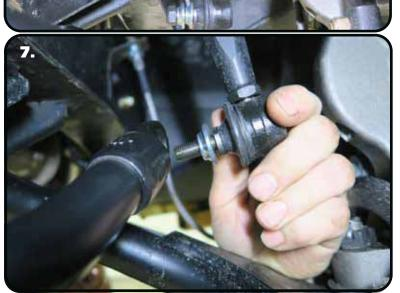
**7.** Remove the nut from the bottom end link. Install a t-bushing on the lower 90 degree end link. The t-bushings are installed with the large diameter against the shoulder of the end link.
