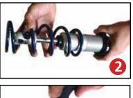
First, using the supplied lower adjuster nut (803-00-199) thread the nut onto the shock from the bottom side as seen in figure 1. Remove the plastic pellet that is in the split of the adjuster nut.
