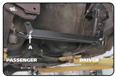
**16.** The centerlink bracket has one attachment hole [A] that is slotted. This is to accommodate the variations in manufacturing and machining processes, as well as any wear that may have occurred to the original centerlink over time. The slot goes on the passenger side centerlink adapter stud.
