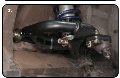
**5.** Place the CoilOver into the coil spring pocket with the stud sticking through the Aluminum upper mount (A). See assembly **Diagram 5**.
