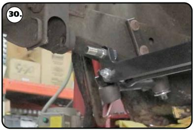
**30.** Install the 5/8"-18 **THIN** mechanical locking nut on the threads of the stud sticking through the centerlink adapter and torque to 45 ftlbs.
