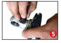
Install upper spring mount retainer clip (803-00-199) into the groove on the upper eyelet as seen in figure 5. Then, reinstall adjuster to complete assembly.
