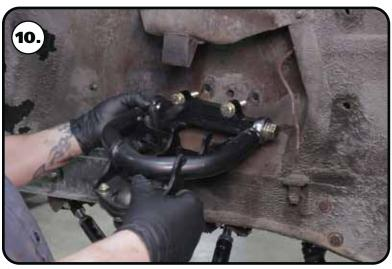
**10.** Bolt the upper StrongArm to the body using  $\frac{1}{2}$ "-13 x 2  $\frac{1}{2}$ " bolts, flat washers and lock washers. The ARROW points to the front of the vehicle. A shim is supplied and may need to be installed between the body and the arms to achieve proper alignment. The arms are preset at the factory so the alignment should be close, but the vehicle must be aligned before driving.
