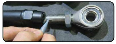
**14d.** Thread the r-joints into the 4-link bar. Thread them in evenly until you achieve the correct center to center length.
