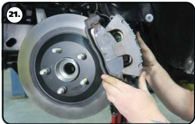
**21.** Install the brake pads and caliper.
