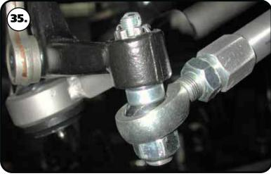
**35.** Install a 5/8"-18 mechanical locking nut. Torque to 45 ftlbs.
