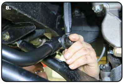
**8.** Insert the 90 degree end link/t-bushing into the swaybar end with the threads pointing toward the engine.
