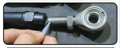
**14d.** Thread the r-joints into the 4-link bar. Thread them in evenly until you achieve the correct center to center length.
