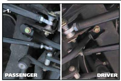
1. The new suspension brace bolts in place of the original brace. Install a 1/2" split lock washer & 1/2" flat washer on each of (2) 1/2"-13 x 1" bolt. Position the crossmember brace at the factory location, behind the lower control arm mount. The bottom of the cross member should angle to the front of the car. Align the mounting holes of the crossmember with the mounting holes in the frame rails. Install a bolt/washer in each of the mounting holes. Torque the crossmember hardware to 50 ftlbs.
