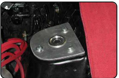
**4.** Lay the Upper Plate on Top of the shock tower with the ShockWave Mount protruding through the large center hole. Line up the the holes in the Upper Plate with the holes drilled in the shock tower and the holes in the ShockWave mount. If the INNER Hole doe not line up, flip the plate over. Install a 5/16" x 1" Flange Bolt in each hole and tighten.
