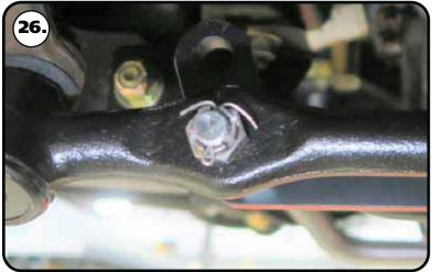
**26.** Torque the nuts to 35 ftlbs and tighten as needed to align cotter pin. Install cotter pin and bend the ends.
