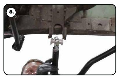
**8.** Install the 2 aluminum spacers into the rod end that goes into the factory control arm pivot. Slip the control arm into the factory frame mount.
