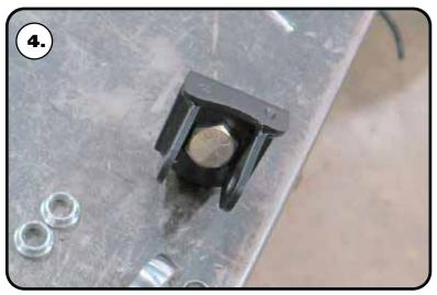
**4.** Insert 3/4"-16 x 2" bolt in the strut rod frame bracket. The head of the bolt needs to be on the side of the bracket with the 2 mounting ears.
