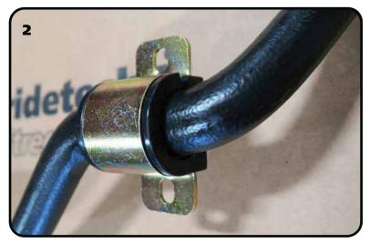
**2.** Install bushing straps over the poly sway bar bushings.
