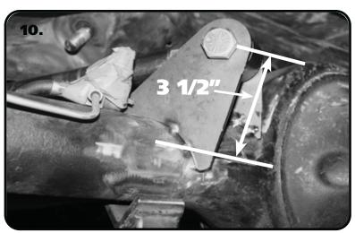
**10.** Refer to Page 8 and set the length of the Upper Bar Jig and install the Tabs on the Jig. Insert the Jig into the Cradle. Set the Upper Tabs on the Rearend. Due to different variations of the Rearend Housings, it may be necessary to modify the tabs for the best fit. The height you are wanting to achieve with the upper bar end is 3 1/2" from the axle center line. Modify the tabs so that the center of the bar bushing will be 3 1/2" from the center of the axle.
