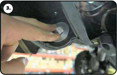
**3.** Test fit the t-bushing in your car's strut rod mount to help determine if the strut rod hole needs buffed out. The t-bushing is installed from the front side of the car.
