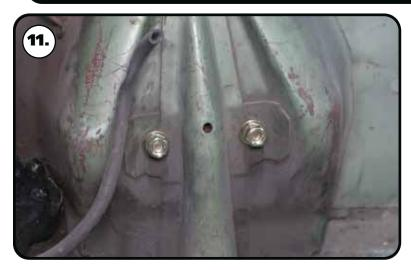
**11.** Install a 1/2" flat washer, 1/2" split lock washer, and 1/2"-13 nut on the threads of the 2 bolts sticking through into the engine compartment. Torque to 75 ftlbs.
