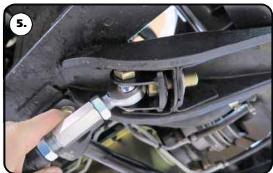
**6.** Insert the 3/4" bolt of the strut rod adapter bracket through the center hole of the t-bushing. The t-bushing and threads of the bolt should be to the front of the car.
