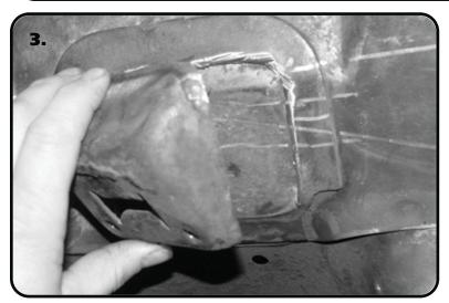
**3.** Remove the Factory Pinion Snubber and Mount from the car. We use a cut off wheel to remove the mount. Notice that we left the mounting lip of the mount attached to the car. This provides another layer of metal for the Front Tab of the Upper Cradle to attach too.
