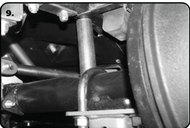
**9.** One helpful trick to maintain ride height when setting the pinion angle is to put a spacer between the axle and the frame. The spacer should be 4 1/2" tall. Set the pinion Angle and axle center. When measuring the axle center you can measure off of the frame rails. We also use a plum bob off the quarter panels to double check the axle center. Refer to Page 7 on Setting the Pinion Angle.
