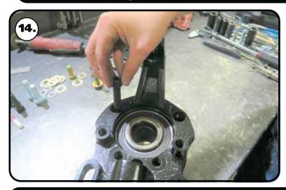
**14.** The Hub is attached to the spindle using (4) M12-1.50 x 40 SHCS. Apply RED Loctite to each of the mounting bolts. Insert them into the correct holes and Torque to 99 ftlbs.
