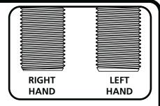
THE 4-LINK BARS, R-JOINTS, AND JAM NUTS HAVE RIGHT HAND AND LEFT HAND THREADS. THIS ALLOWS THE BAR TO BE ADJUSTED WITHOUT REMOVING IT. THE HEX END OF THE BAR IS LEFT HAND THREAD. THE LEFT HAND JAM NUT HAS AN COUNTER-CLOCKWISE ARROW STAMPED INTO IT. IMAGE 3 WILL HELP YOU DETERMINE THE THREADS OF THE R-JOINTS.
