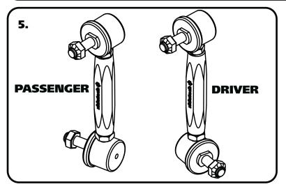
**5.** The driver and passenger sway bar linkages are clocked opposite of each other. With the top stud pointing toward you, the stud on the lower should be pointing to the right for the driver side, to the left for the passenger side. Using **Diagram 5** as a reference, set the linkage to 6" center to center. Snug the jam nuts against the center adapter.
