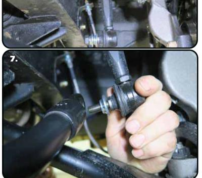
**7.** Remove the nut from the bottom end link. Install a t-bushing on the lower 90 degree end link. The t-bushings are installed with the large diameter against the shoulder of the end link.
