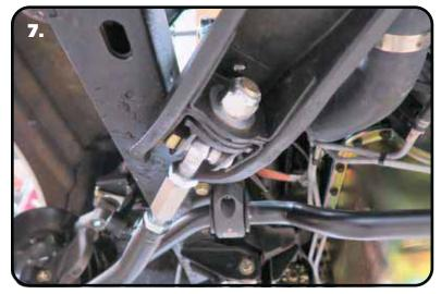
**7.** Install a 3/4"-16 nylok nut on the threads of the bolt sticking through the t-bushing. Torque to 120 ftlbs.
