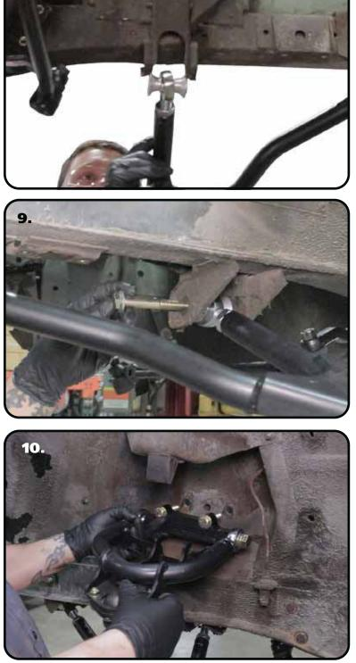
**8.** Install the 2 aluminum spacers into the rod end that goes into the factory control arm pivot. Slip the control arm into the factory frame mount.
