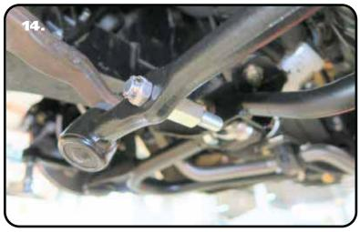
**14.** The studs with the long hex on them will get installed into the factory centerlink with the taper going into the centerlink, a 7/16" castle nut is used to attach it to the centerlink. The straight shank will point to the front of the car.
