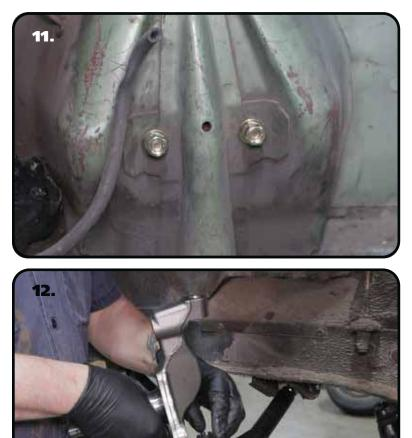
**11.** Install a 1/2" flat washer, 1/2" split lock washer, and 1/2"-13 nut on the threads of the 2 bolts sticking through into the engine compartment. Torque to 75 ftlbs.
