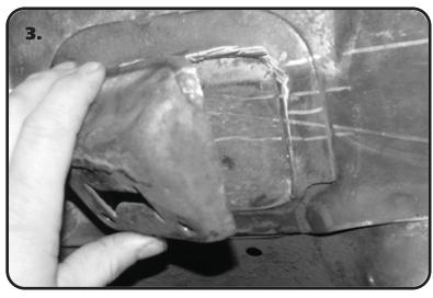
**3.** Remove the Factory Pinion Snubber and Mount from the car. We use a cut off wheel to remove the mount. Notice that we left the mounting lip of the mount attached to the car. This provides another layer of metal for the Front Tab of the Upper Cradle to attach too.
