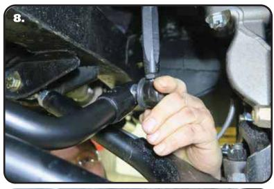
**8.** Insert the 90 degree end link/t-bushing into the swaybar end with the threads pointing toward the engine.
