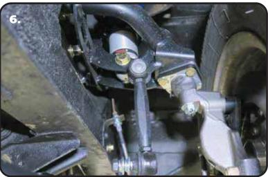
**6.** Remove the nut from the top end link. Insert the stud of the end link in the tab of the upper control arm with the stud pointing to the rear of the car. The lower stud should be pointing toward the engine. Install the nut on the stud of the end link and torque to 37 ftlbs. Repeat on the second side.
