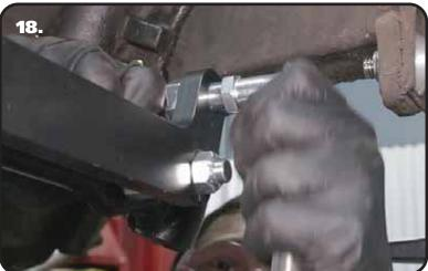
**18.** The studs with the short hex get installed into the centerlink adapter. The short side goes into the adapter attached with the 5/8"-18 thin top lock nut, with the long side of the stud pointing forward.
