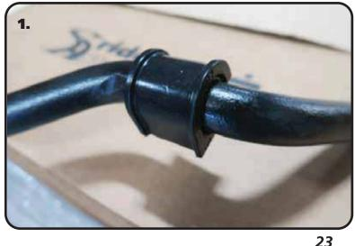
**1.** Open the sway bar bushing at the split and slip it **OVER** the sway bar. Do this for both bushings.
