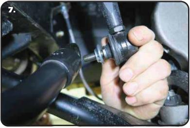
**7.** Remove the nut from the bottom end link. Install a t-bushing on the lower 90 degree end link. The t-bushings are installed with the large diameter against the shoulder of the end link.
