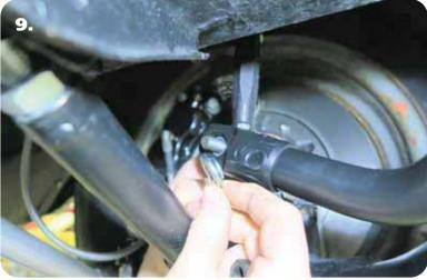
**9.** Install a 2nd t-bushing with the small diameter into the swaybar. Install the nut and torque to 37 ftlbs. Do this for both sides.
