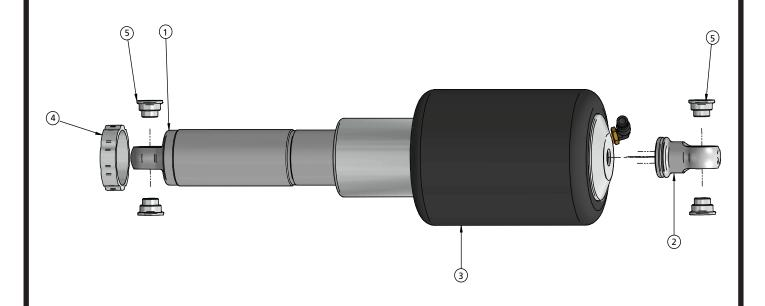
WARNING: ATTEMPTING TO REMOVE THE AIR FITTING WILL DAMAGE IT AND VOID THE WARRANTY.
