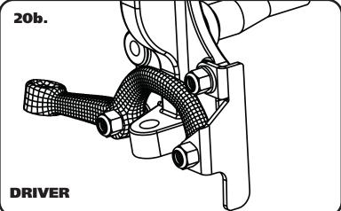
**20a.** Install the steering arms and steering stops onto the spindle using **Images 20a & 20b** as a reference. The steering arms angle toward the centerlink, and the tie rod mounting holes are to the rear of the car. The steering stops are marked D and P.
