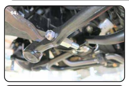
**14.** The studs with the long hex on them will get installed into the factory centerlink with the taper going into the centerlink, a 7/16" castle nut is used to attach it to the centerlink. The straight shank will point to the front of the car.
