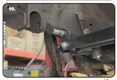
**19.** Install the 5/8"-18 **THIN** mechanical locking nut on the threads of the stud sticking through the centerlink adapter and torque to 45 ftlbs.
