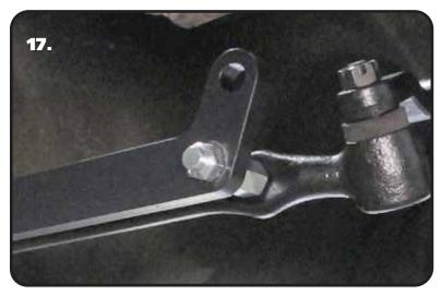
**17.** Install the 1/2"-20 mechanical locking nuts and torque to 50 ftlbs.
