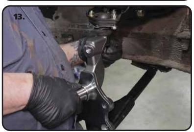
**13.** Install the spindle on the upper ball joint pin. Torque the ball joint castle nut to 50 ftlbs and tighten to align the cotter pin holes. Install the cotter pin in the ball joint pin hole and bend the ends of the cotter pin to hold it in place. Install the grease zerk supplied with the ball joint.
