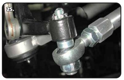
**25.** Install a 5/8"-18 mechanical locking nut. Torque to 45 ftlbs.
