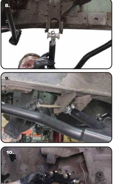
8. Install the 2 aluminum spacers into the rod end that goes into the factory control arm pivot. Slip the control arm into the factory frame mount.
