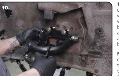
**10.** Bolt the upper StrongArm to the body using  $\frac{1}{2}$ "-13 x 2  $\frac{1}{2}$ " bolts, flat washers and lock washers. The ARROW points to the front of the vehicle. A shim is supplied and may need to be installed between the body and the arms to achieve proper alignment. The arms are preset at the factory so the alignment should be close, but the vehicle must be aligned before driving.
