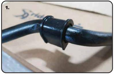
**1.** Open the sway bar bushing at the split and slip it **OVER** the sway bar. Do this for both bushings.
