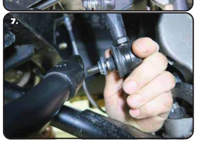
**7.** Remove the nut from the bottom end link. Install a t-bushing on the lower 90 degree end link. The t-bushings are installed with the large diameter against the shoulder of the end link.
