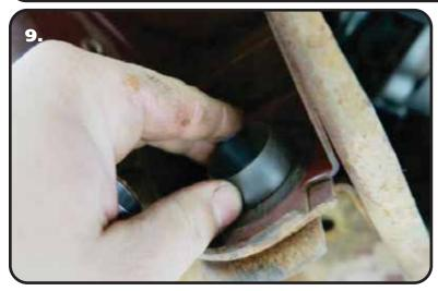
**9.** Refer to **(Figure 10)** for the Delrin Strut Rod Bushing assembly order. The Delrin Strut Rod Bushing will insert into the frame bushing hole with the rounded side of the bushing outward. A Bushing needs to be installed on both the front and rear side of the frame. With a Delrin Strut Rod Bushing on each side of the frame, insert the INNER Sleeve in the Bushings. This will help hold them in place.
