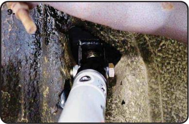
**9.** The Shock is mounted in the Upper Mount with the BODY UP. It is held in place with a 1/2"-20 x 2 1/4" Hex Bolt & 1/2"-20 Nylok. If the threads of the bolt would happen to touch the floor pan of the car, a 1/2" Flat Washer can be installed under the head of the bolt.
