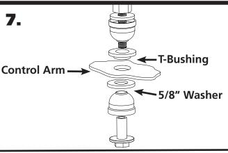
7. Install the End Links using **Diagram 8** as a reference. Insert the SMALL diameter of the 5/8" ID t-bushing into the stock sway bar hole of the lower control arm. A 5/8" washer goes on the bottom side of the control arm. Tighten the end link barrel nut until it is flush with the end of the bolt, and then tighten it 2 more complete rounds.
