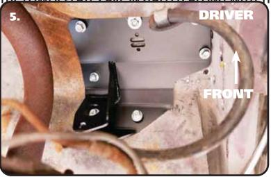
the top of the shock to behind the axle. The Mount nests in the car one way. Position the Mount in the car with the Shock attaching point to the rear and away from the frame. The outside edge of the mount will touch the frame with the front edge against a body seam. Using these points as a guide, the Mount will fit the contours of the body. With the Mount in position, use it to mark the 7 holes and drill them 5/16"
