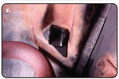
7. Install the Passenger Shock Mount will be installed in the OEM location. The Shock Mount is shaped to fit the body and will only fit into the OEM location one way. Install the mount into the OEM location with the Stud sticking through the OEM shock hole. Have someone hold the mount in place while installing the top support and mounting hardware,
