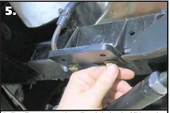
**5.** The offset mounting plate will get bolted to the OEM sway bar mount. It is bolted to the OEM holes using the SLOTTED holes in the offset plate with the (2) round holes offset toward the engine. Install a 3/8" flat washer on (2) 3/8"-16 x 1 1/4" hex bolts. A bolt/ washer will go in each of the (2) mounting holes. Insert a bolt/ washer through each slotted hole and OEM mounting hole. With the bolt/washers installed, install a 3/8" flat washer on the threads followed by a 3/8"-16 nylok nut.
