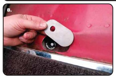
**8.** Insert the Upper Backer through the shock access hole. Install it with the Stud from the Shock Mount sticking through the hole in the Backer. Rotate the Backer on the Stud to get it sitting flat against the body of the car. Once the Backer is positioned properly, install a 7/16" Flat Washer and 7/16"-14 Nylok Nut on the Stud and tighten. Make sure the Shock Mount stays positioned correctly while tightening.
