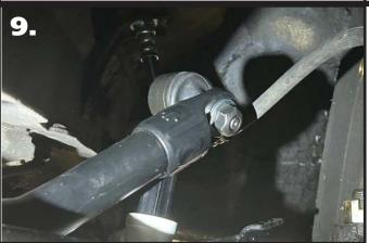
9. Insert the 90 degree end link/t-bushing into the swaybar end with the threads pointing toward the WHEEL. Install a 2nd t-bushing with the small diameter into the swaybar. Install the nut and torque. Do this for both sides.
