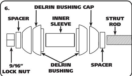
**8**. Install a Spacer on the strut rod followed by the Delrin Bushing Cap. Insert the strut rod through the Bushing Sleeve until the Ball is nested into the Bushing Cap. Install a second Bushing Cap on the strut rod followed by a 2nd Spacer. Next, install a 9/16" Lock Nut on the threads of the strut rod. Install the OEM castle nut on the end of the strut rod with a cotter pin through it.
