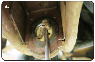
**6.** A Delrin Bushing setup for the strut rod is also included in this kit. The liner that is installed in the frame hole has to be removed. Use a chisel to distort it and remove it. In **(Figure 4)** we distorted it from the bottom edge and removed it.
