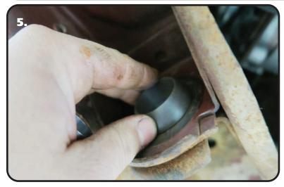
7. Refer to (Figure 6) for the Delrin Strut Rod Bushing assembly order. The Delrin Strut Rod Bushing will insert into the frame bushing hole with the rounded side of the bushing outward. A Bushing needs to be installed on both the front and rear side of the frame. With a Delrin Strut Rod Bushing on each side of the frame, insert the INNER Sleeve in the Bushings. This will help hold them in place.
