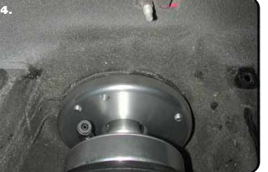
**4.** Hold the aluminum upper mount agianst the bottom of the shock tower lining up the threaded holes with the holes drilled out in the shock tower.
