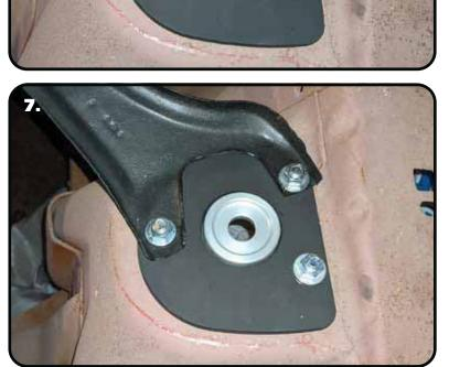
**7.** Install the export brace on the bolts sticking through the top plate. Install a 3/8" SAE flat washer & 3/8"-16 nylok nut on the threads of each of the bolts. Torque the nylok nuts to 15 ft-lbs.
