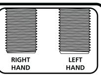
THE 4-LINK BARS, R-JOINTS, AND JAM NUTS HAVE RIGHT HAND AND LEFT HAND THREADS. THIS ALLOWS THE BAR TO BE ADJUSTED WITHOUT REMOVING IT. THE HEX END OF THE BAR IS LEFT HAND THREAD. THE LEFT HAND JAM NUT HAS AN COUNTER-CLOCKWISE ARROW STAMPED INTO IT. IMAGE 3 WILL HELP YOU DETERMINE THE THREADS OF THE R-JOINTS.
