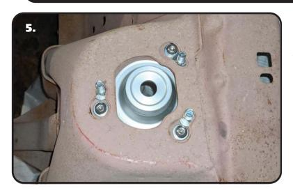
**5.** Install a 5/16" split lock washer & 5/16" SAE flat washer on each of (3) 5/16"-18 x 1" button head cap screws. Apply red loctite to the threads of each of the bolts. Hold the lower mount in poistion and thread the mounting bolts into the (3) mounting holes. Torque the bolts to 13 ft-lbs.
