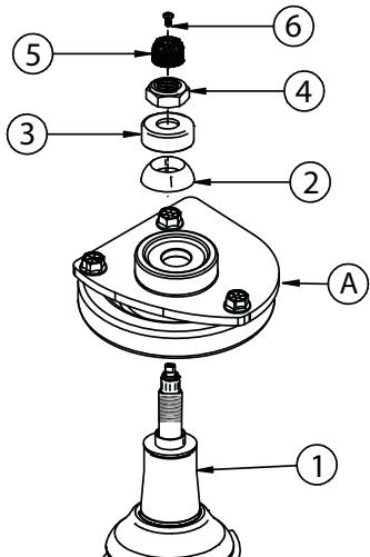
**9.** Place the CoilOver into the coil spring pocket with the stud sticking through the Aluminum upper mount (A). See assembly **Diagram 9**.
