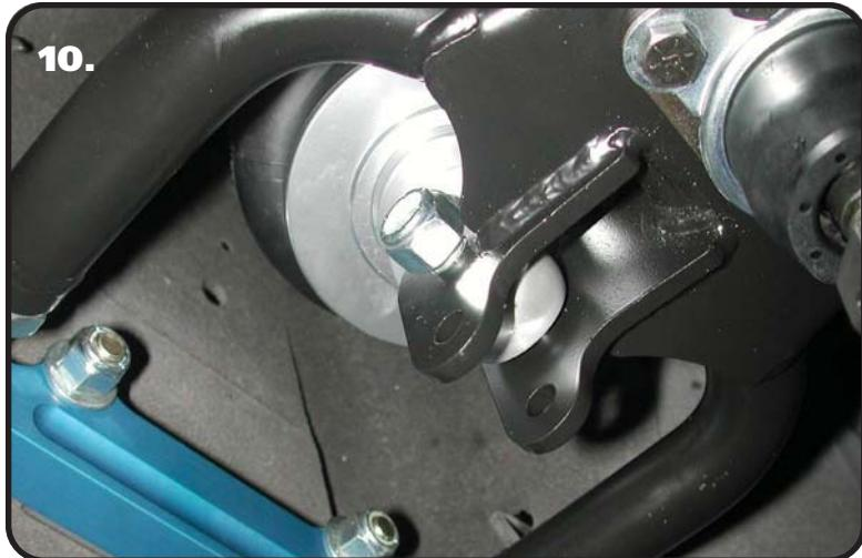
**10.** Install the a Bearing Spacer in each side of the Bearing. The SMALL part of the spacer inserts into the Inside Diameter of the shock bearing. Raise the lower arm up to the CoilOver and bolt them together using the 1/2" x 2 1/4", & Nylok Nuts supplied with the StrongArms. Torque to 50 ftlbs.
