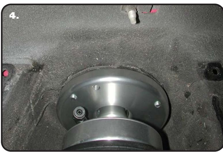
4. Hold the aluminum upper mount agianst the bottom of the shock tower lining up the threaded holes with the holes drilled out in the shock tower.
