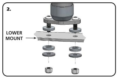
**2. (Image 2)** shows the assembly of the lower shock bushings. Install a Bushing on the each of threads protruding through the lower shock plates.
