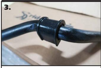
**3.** Open the sway bar bushing at the split and slip it **OVER** the sway bar. Do this for both bushings.
