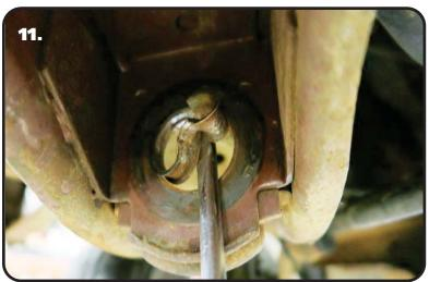
**11.** A Delrin Bushing setup for the strut rod is also included in this kit. The liner that is installed in the frame hole has to be removed. Use a chisel to distort it and remove it. In **(Image 11)** we distorted it from the bottom edge and removed it.
