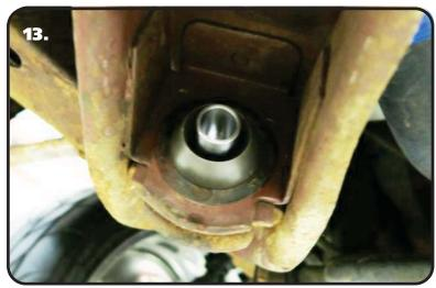
**13.** Install the Inner Sleeve in the Strut Rod Bushings. Center the Sleeve in the Bushings, this will also help hold the Bushings in place during reassembly of the strut rod.
