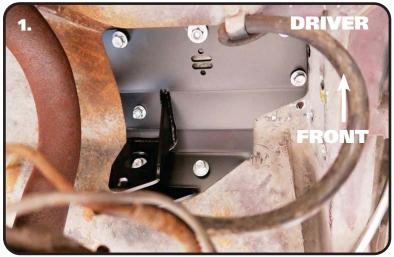
1. The Driver Upper Shock Mount repositions the top of the shock to behind the axle. The Mount nests in the car one way. Position the Mount in the car with the Shock attaching point to the rear and away from the frame. The outside edge of the mount will touch the frame with the front edge against a body seam. Using these points as a guide, the Mount will fit the contours of the body. With the Mount in position, use it to mark the 7 holes and drill them 5/16"
