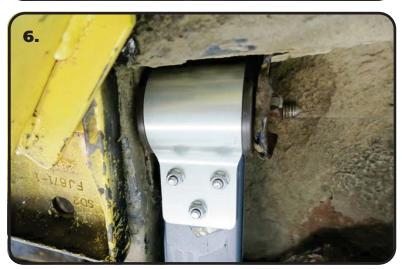
**6.** Swing the Leaf Spring up and attach the **LARGE BUSHING END** of the Composite Leaf Spring into the OEM front leaf spring mount using a 1/2"-13 x 4.5" Hex Bolt and 1/2"-13 Nylok Nut.
