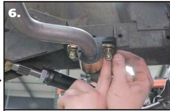
**6.** Install the sway bar in position in the car. The center of the bar should be to the front of the car. The outer arms of the sway bar will bend upward. Install a 3/8" flat washer on (4) 3/8"-16 x 1 1/4" hex bolts. A bolt/washer will go in each of the 4 mounting holes. With the bolt/washers installed, install a 3/8" flat washer on the threads followed by a 3/8"-16 nylok nut. Do **NOT** completely tighten the hardware. It will be left partially loose until the end links are installed.
