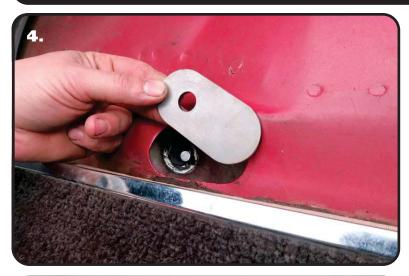
**4.** Insert the Upper Backer through the shock access hole. Install it with the Stud from the Shock Mount sticking through the hole in the Backer. Rotate the Backer on the Stud to get it sitting flat against the body of the car. Once the Backer is positioned properly, install a 7/16" Flat Washer and 7/16"-14 Nylok Nut on the Stud and tighten. Make sure the Shock Mount stays positioned correctly while tightening.
