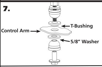
7. Install the End Links using **Diagram 7** as a reference. Insert the SMALL diameter of the 5/8" ID t-bushing into the stock sway bar hole of the lower control arm. A 5/8" washer goes on the bottom side of the control arm. Tighten the end link barrel nut until it is flush with the end of the bolt, and then tighten it 2 more complete rounds.
