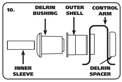
**10.** Install the Outer Shell into the control arm. Next, install the Delrin Bushing into the Outer Shell followed by the Inner Sleeve. With the Delrin Bushing and Inner Sleeve installed, install the Delrin Spacer over the SMALL end of the Delrin Bushing. The ROUNDED surface will be out, away from the control arm.
