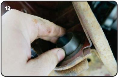
**11.** Refer to **(Image 14)** for the Delrin Strut Rod Bushing assembly order. The Delrin Strut Rod Bushing will insert into the frame bushing hole with the rounded side of the bushing outward. A Bushing needs to be installed on both the front and rear side of the frame.
