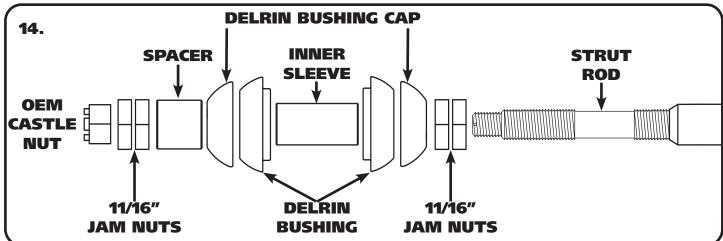
**15**. Install (2) 11/16" Jam Nuts on the INNER THREADS of the strut rod followed by the Delrin Bushing Cap. Insert the strut rod through the Bushing Sleeve until the Ball is nested into the Bushing Cap. Install a second Bushing Cap on the strut rod followed by the Spacer. Next, install the (2) 11/16" Jam Nuts on the OUTER THREADS. Install the OEM castle nut on the end of the strut rod with a cotter pin through it. Position isn't critical, it will be adjusted when the front end is aligned.
