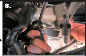
**8.** Install a T-Bushing on each of the 90 degree end links. The t-bushings are installed with the large diameter against the shoulder of the end link.
