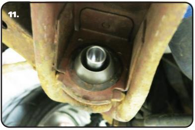
**11.** Install the Inner Sleeve in the Strut Rod Bushings. Center the Sleeve in the Bushings, this will also help hold the Bushings in place during reassembly of the strut rod.
