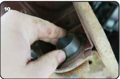
**10.** Refer to **(Figure 12)** for the Delrin Strut Rod Bushing assembly order. The Delrin Strut Rod Bushing will insert into the frame bushing hole with the rounded side of the bushing outward. A Bushing needs to be installed on both the front and rear side of the frame.
