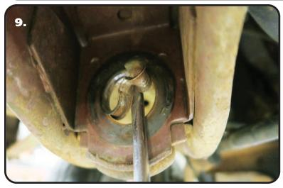
**9.** A Delrin Bushing setup for the strut rod is also included in this kit. The liner that is installed in the frame hole has to be removed. Use a chisel to distort it and remove it. In **(Figure 9)** we distorted it from the bottom edge and removed it.
