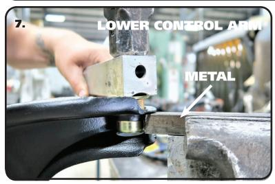
7. Remove the OEM Lower Control Arm Bushings. This Kit contains 2 different sizes of Lower Control Arm Bushings. Use your control arm to determine which size is needed. Use (Figure 8) to help with determine the Bushing assembly order. Support the back side of the Flange the Bushing is being Installed in. Use a piece of metal clamped in a Bench Vise for the Lower Control Arms.
