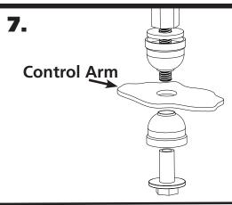
**7.** Install the End Links using **Diagram 7** as a reference. Tighten the end link barrel nut until it is flush with the end of the bolt, and then tighten it 2 more complete rounds.
