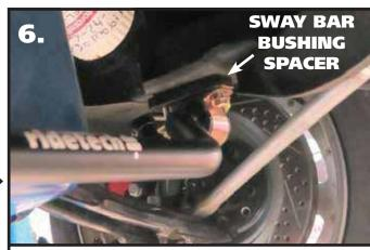
**6.** Install a 3/8" flat washer on each of the (4) 3/8" x 1 1/2" bolts. The sway bar bushing spacer will be installed between the sway bar bushing and frame. Push the bar up to the frame, installing the spacer in place. Hold it in position and install (2) bolt/washers in each side. Install a 3/8" flat washer & 3/8" nylok nut on the bolts and snug the hardware.
