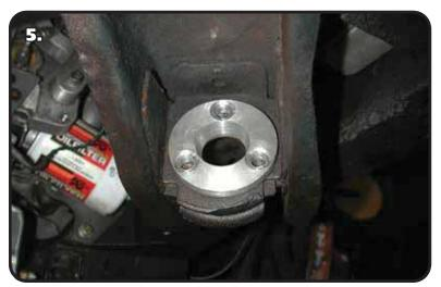
**5.** Using the bearing retainer as a template; drill three 3/8" holes in the frame to secure the assembly. Use three 3/8" x 1  $\frac{1}{4}$ " SHCS and lock washers to secure the assembly. Torque to 30 ft-lbs.
