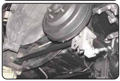
**8.** Install the Lower Bars. The Front Lower uses the WIDE(70013767) R-Joint Spacers inserted into each side of the R-Joint. The Axle end of the bar gets a NARROW(70013334) R-Joint Spacer inserted into each side of the R-Joint. The bar is attached to the Axle Mount in the **TOP HOLE** using (1) 5/8" x 2 3/4" Hex Bolt, and (1) 5/8" Thin Nylok Jam Nut. The front of the Lower Bar is attached with 1/2"x 6" Hex Bolt(64-67) or 1/2"x 4 1/2"Hex Bolt(68-70), and (1) 1/2" Nylok Nut.
