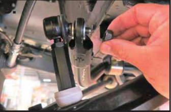
**9.** Insert the 90 degree end link/t-bushing into the swaybar end with the threads pointing toward the engine. Install a 2nd t-bushing with the small diameter into the swaybar. Install the nut and torque. Do this for both sides.
