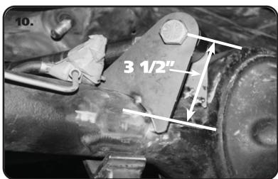
**10.** Refer to Page 7 and set the length of the Upper Bar Jig and install the Tabs on the Jig. Insert the Jig into the Cradle. Set the Upper Tabs on the Rearend. Due to different variations of the Rearend Housings, it may be necessary to modify the tabs for the best fit. The height you are wanting to achieve with the upper bar end is 3 1/2" from the axle center line. Modify the tabs so that the center of the bar bushing will be 3 1/2" from the center of the axle
