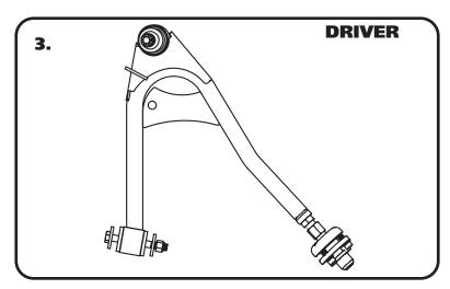
**3.** The control arms are marked "D" for Driver and "P" for Passenger. The control arms will be installed in the car with the ball joint pin pointing up.
