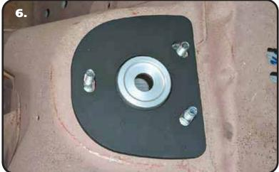
**6.** Lay the upper plate on top of the shock tower with the ShockWave mount protruding through the large center hole.
