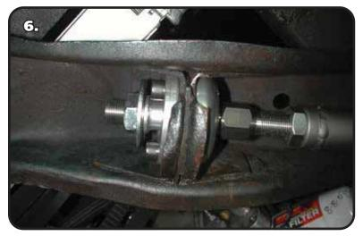
**6.** Slide the stud through the bearing, then slide the aluminum spacer over the stud with the larger end toward the front of the car. Secure the assembly with a ¾" Nylok Nut and flat washer. Use **Images 6 & 7** as a guide.
