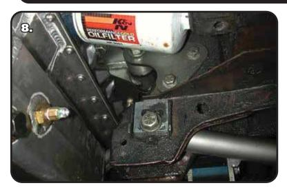
**8.** Eccentric eliminator plates are included, one must be installed on each side of the frame. Start out with it in the center, make sure both plates are in the same position. Attach the other end of the lower control arm to the factory frame mount using a ½" x 4 ½" bolt and Hex nut. Torque to 75 ft-lbs.
