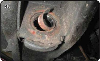
**4**. Be sure to remove the outer bushing sleeve from the strut rod frame mount.
