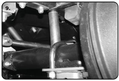
**9.** One helpful trick to maintain ride height when setting the pinion angle is to put a spacer between the axle and the frame. The spacer should be 4 1/2" tall. Set the pinion Angle and axle center. When measuring the axle center you can measure off of the frame rails. We also use a plum bob off the quarter panels to double check the axle center. Refer to Page 6 on Setting the Pinion Angle.
