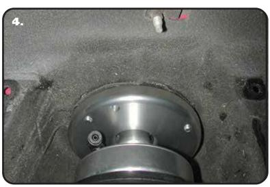
**4.** Hold the aluminum upper mount agianst the bottom of the shock tower lining up the threaded holes with the holes drilled out in the shock tower.
