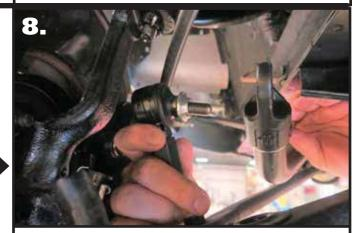
**8.** Install a T-Bushing on each of the 90 degree end links. The t-bushings are installed with the large diameter against the shoulder of the end link.
