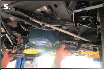
**5.** Install the sway bar in position in the car. The center of the bar should be to the front of the car. The outer arms of the sway bar will bend upward. Use **Picture 6** as a reference.
