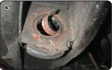
**4**. Be sure to remove the outer bushing sleeve from the strut rod frame mount.
