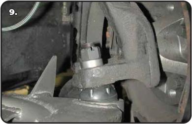
**10.** Lubricate control arm bushing with Lithium grease.
