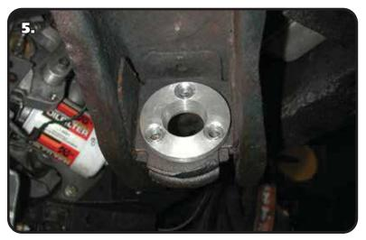
**5.** Using the bearing retainer as a template; drill three 3/8" holes in the frame to secure the assembly. Use three 3/8" x 1 ¼" SHCS and lock washers to secure the assembly. Torque to 30 ft-lbs.
