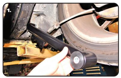
The kit comes with the 12mm inner sleeves installed. If your car has 14mm bolts in the lowers, you will need to switch the inner sleeves.
