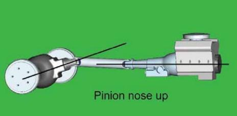
How do you set the pinion angle? On a single-piece shaft you want to set it up where a line drawn through the center of the engine crankshaft or output shaft of the transmission and a line drawn through the center of the pinion are parallel to each other but not the same line.
