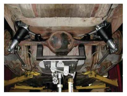
16. Bolt the axle tabs to the upper bar jig using a 5/8" x 2 3/4" bolt and nyloc as shown in the picture. The upper bar should measure 12" C-C.
