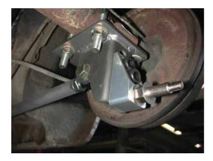
10. The 63-64 years use a 3/4" bolt, it will be replaced with the 9/16" x 4  $\frac{1}{2}$ " bolt supplied in the kit. The bolt hole in the frame will need to be drilled out to 9/16". The Front Lower uses the WIDE(70013768) R-Joint Spacers inserted into each side of the R-Joint with the LARGE Aluminum T-bushing in the leaf spring hole.
