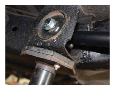
8. The 60-62 years use a 9/16" bolt, it will be reused to attached the lower bars. The Front Lower uses the WIDE(70013768) R-Joint Spacers inserted into each side of the R-Joint.
