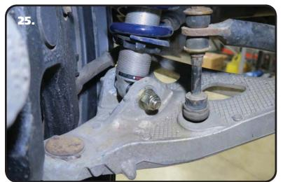
**25.** Install a 5/8" flat washer and 5/8-18" nylok nut on the threads of the bolt that are sticking out of the rear control arm tab. Torque to 115 ftlbs.
