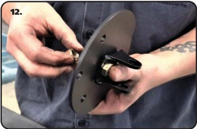
**12.** Insert a 1/2"-13 x 1 1/12" bolt through each hole of the flange/mount. The bolts need to be installed with the bolt head in the upper bracket. Refer to **Images 12 & 13**.
