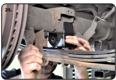
**25.** Position the Flip Bracket on the locating pins. Again, the locating pin holes go to the front of the truck.
