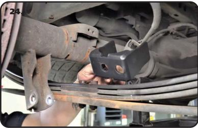
**24.** The Flip Bracket is positioned on the leaf spring locating pins. the locating pin holes will need to be positioned to the front of the truck.
