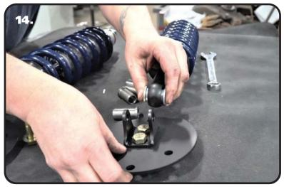
**14.** Install the 1/2" I.D. bearing spacers into the bearing in the shock eyelet. These spacers have a through hole that is 1/2" diameter. The small diameter of the spacers will insert into the shock bearing.
