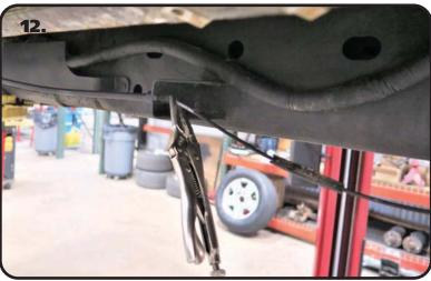
12. The emergency brake cables will need to be disconnected to flip the leaf springs under the axle. The emergency brake needs to be off to unhook the cable. The emergency brake cable will need to be disconnected to allow the leaf springs to be moved under the rear differential. Pull out on the cable. It should pull out of the sheath that goes to the front of the truck. With the cable pulled out, clamp the cable right where it goes into the forward sheath.
