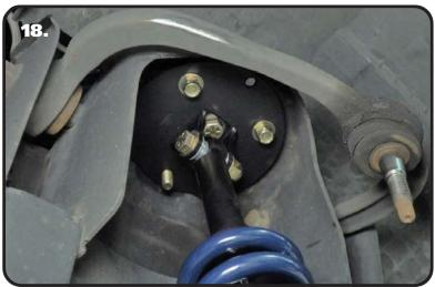
**18.** Install a 7/16" flat washer on each of (3) 7/16"-14 x 1 1/4" hex bolts. Install the bolt/ washer in the frame/mount from the top side with the threads pointing down. Install a 7/16" flat washer and 7/16"-14 nylok nut on the threads of each bolt sticking through the frame. Torque the hardware to 50 ftlbs. Repeat steps 11-18 on the remaining side.
