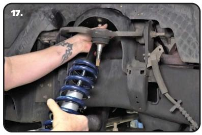
**17.** Position the mount/coilover in the truck. It will be placed in the OEM location. Line up the locating hole and 3 mounting holes.
