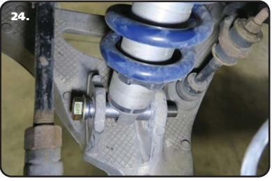
**24.** Install a 5/8" flat washer on a 5/8"-18 x 5" hex bolt. Insert the bolt in from the front side with the threads to the rear of the truck. Insert it through the t-bushings and shock bearing.
