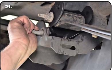
21. Insert the Shackle into the leaf spring hanger. Line up the holes in the hanger with the inner sleeve of the shackle. Install a 9/16" flat washer on a 9/16"-18 x 5" hex bolt. Insert the bolt/washer through the frame and shackle. Install a 9/16" flat washer and 9/16"-18 nylok nut on the threads of the bolt. Do not tighten the hardware at this time.
