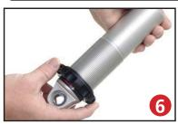
First, using the supplied lower adjuster nut (803-00-199) thread the nut onto the shock from the bottom side as seen in figure 6. Remove the plastic pellet that is in the split of the adjuster nut.
