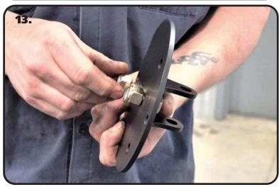
**13.** Install a 1/2"-13 nylok nut on the threads of each bolt that is sticking through the mount. Torque to 75 ftlbs.
