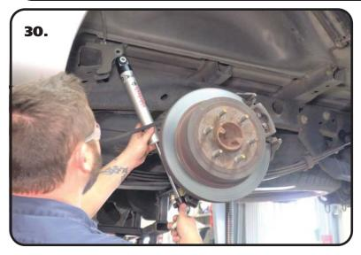
**30.** Install the BODY of the shock in the OEM frame mount using the OEM hardware.
