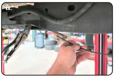
**13.** Disconnect the rear cable from the front cable at the connector. This is done by sliding the rear cable forward in the connector.
