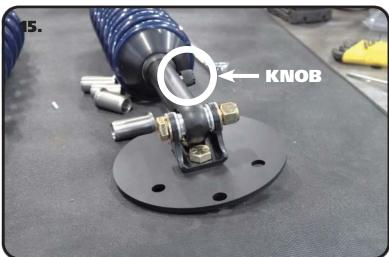
15. Insert the shock eyelet into the upper mount. Install each CoilOver in the upper mount with the Adjusting Knob on opposite sides of each other. Line up the shock bearing/spacers hole with the mounting holes of the upper mount. Install a 1/2" flat washer on a 1/2"-13 x 2 3/4" bolt. Insert a bolt/washer through the mount/shock. Install a 1/2" flat washer and 1/2"-13 nylok nut on the threads of the bolt that are sticking through the mount. Torque the upper mounting hardware to 75 ftlbs.
