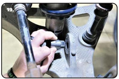
**19.** Insert the T-Bushing (90001382) into the front side of the REAR TAB of the OEM shock mount. The REAR TAB IS THE THICKER TAB. This T-bushing is Tapered on the CoilOver side. Insert the small OD into the control arm with the taper away from the control arm.
