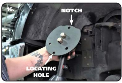
**16.** The upper mount has 4 holes in the perimeter of the flange. 3 of these holes are mounting holes, 1 is a locating hole. The flange is also notched out on the side opposite of the locating hole. The upper mount needs to be installed in the truck with the locating hole toward the wheel of the truck. The notch will be to the frame.
