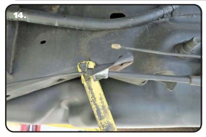
**14.** Disconnect the passenger side cable from the bracket that is made into the driver side emergency brake cable.
