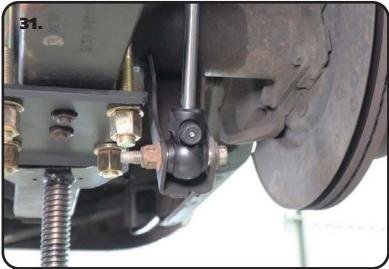
**31.** Attach the EYELET of the Shock in the OEM mount that is on the axle housing. Attach the shock using the OEM hardware. Position the Shock with the Adjuster Knob pointing out, away from the axle.
