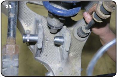
**21.** The kit includes a 2nd T-bushing (90001383) that has a long straight OD. This bushing goes in from the front side of the front tab of the OEM shock mount. The larger OD at the very end will be to the front of the truck.
