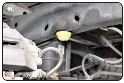
**11.** Install the supplied bump stops by threading them into the previously installed u-nut.
