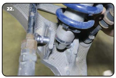
**22.** You will need to jack up the lower control arm to do the next few steps. Jack up the control arm until the bottom bearing of the coilover is aligned with the rear t-bushing.
