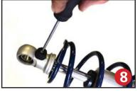
Before the upper spring mount can be installed screw the adjuster knob on the upper eye mount to the firmest setting (clockwise) as seen in figure 8. Then remove the Knob by holding it while removing the center screw.
