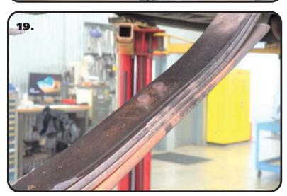
**19.** Remove the locating pins from the leaf spring pack. Reinstall the locating pins from the TOP side. Reinstall the nuts on the BOTTOM side and tighten. With the nuts tight, remove the clamps. Repeat on the second spring.
