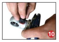
Install upper spring mount retainer clip (803-00-199) into the groove on the upper eyelet as seen in figure 10. Then, reinstall adjuster to complete assembly.
