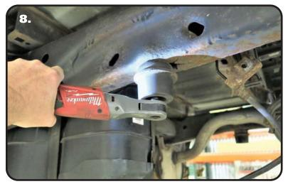
**9.** The OEM bump stop mount will need to be removed.
