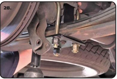
THE ARROW ON THE BRACKET SHOULD POINT TO THE FRONT OF THE TRUCK. Hold the Leaf Spring Bracket in place and install a 5/8" Flat Washer & 5/8"-18 High Nut on the threads of the u-bolts. Snug the nuts down evenly and tighten them in a criss-cross fashion to 130 ftlbs.
