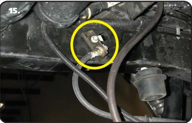
**15.** Unbolt the brake line bracket from the inside of the drivers side frame rail. This will help provide enough slack in the lines to be able to flip the leaf springs on the bottom side of the axle. Retain the hardware, this bracket will be reinstalled later.
