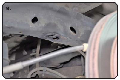
**10.** Remove the OEM u-nut from the frame and replace it with the 3/8"-16 u-nut supplied in the kit.
