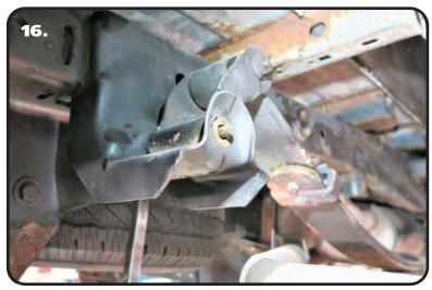
**16.** Remove the rear shackle from the hanger. After removing the shackle from the hanger, remove the shackle from the leaf spring.
