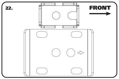
**22.** The Flip Kit has the locating holes offset to center the wheel in the wheel opening. **Image 22** illustrates a top view of the Flip Bracket and the Leaf Spring Plate. Notice the HOLES are offset to the FRONT of the truck. The ARROW in the plate needs to point to the front of the truck.
