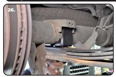
**26.** Slowly lower the axle into the Flip Bracket, making sure the tabs go up into the leaf spring saddle. THE FLIP BRACKET WILL POSITION THE PINION AT THE CORRECT ANGLE.
