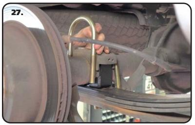
**27.** Slip the U-Bolts over the axle tube with the threads pointing down.
