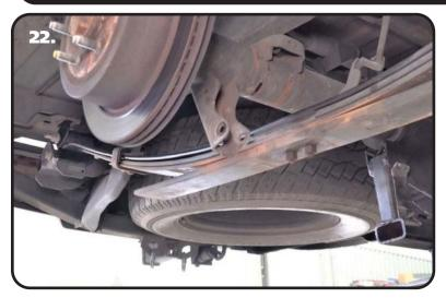
**23.** Raise the axle high enough to get the Flip Bracket positioned on the leaf spring.
