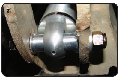
7. With the **WIDE** spacers installed in the lower ShockWave Bearing, insert the ShockWave into the Lower Control Arm. Align the hole in the ShockWave with the hole in the T-bushing. Insert the 1/2" x 3 3/4" Hex Bolt into the mounting hole in Lower Control Arm. Install a 1/2" Nylok Nut onto the Bolt and tighten.
