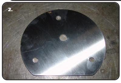
**2.** Both sides of the suspension use the same Upper Mounting Plate. Both Upper Mounting Plates and Shock Mounts are assembly identically to each other. Figure "2" shows the bottom side of the Mounting Plate.
