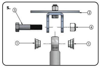
**5.** Install the Air Fitting into the ShockWave using a thread sealant on the fitting threads. Insert the **NARROW** upper spacers(1) into the upper shock bearings. Install the **WIDE** spacers into the Lower Shock Bearing. With the spacers installed insert the ShockWave assembly into the upper shock mount(2). Align the holes in the bracket with the hole in the Shock spacers and insert the 1/2 x 2 1/2"" Bolt(3) and secure with the 1/2" Nylok Nut(4).
