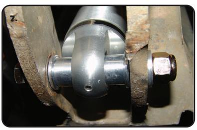
7. With the **WIDE** spacers installed in the lower CoilOver Bearing, insert the CoilOver into the Lower Control Arm. Align the hole in the CoilOver with the hole in the T-bushing. Insert the 1/2" x 3 3/4" Hex Bolt into the mounting hole in Lower Control Arm. Install a 1/2" Nylok Nut onto the Bolt and tighten.
