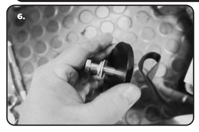
**6.** Install a 3/8" Split Lock Washer, followed by a 3/8" Flat Washer, on the 3/8"-16 x 1 1/2" Hex Bolt. Insert the Bolt into the hole in the Clamping Plate.
