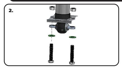
**2.** Attach the Trunnion to the OEM Control arm using the supplied Hardware. It may be necessary to rotate the Trunnion to get it in the correct position. This can be done by sticking a screwdriver in one of the slots and spinning the trunnion in the shock bushing. Torque the hardware to 17ftlbs. Do this for both sides. Reattached the sway bar linkage.
