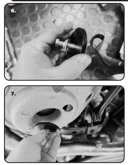
**6.** Install a 3/8" Split Lock Washer, followed by a 3/8" Flat Washer, on the 3/8"-16 x 1 1/2" Hex Bolt. Insert the Bolt into the hole in the Clamping Plate.
