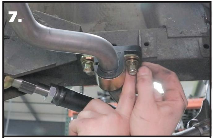
**7.** Install the sway bar in position in the car. The center of the bar should be to the front of the car. The outer arms of the sway bar will bend upward. Install a 3/8" flat washer on (4) 3/8"-16 x 1 1/4" hex bolts. A bolt/washer will go in each of the 4 mounting holes. With the bolt/washers installed, install a 3/8" flat washer on the threads followed by a 3/8"-16 nylok nut. Do **NOT** completely tighten the hardware. It will be left partially loose until the end links are installed.
