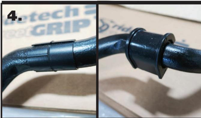
4. Open the delrin liner at the split and slip it over the swaybar. Position it in the area that the bushing will ride based on the location of the stock swaybar. Do this on both ends of the swaybar. Next, open the swaybar Bushing at the split and slide it **OVER** the delrin liner. Do this on both delrin liners.
