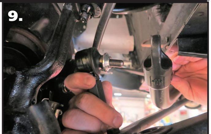
**9.** Install a T-Bushing on each of the 90 degree end links. The t-bushings are installed with the large diameter against the shoulder of the end link.
