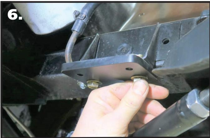
**6.** The offset mounting plate will get bolted to the OEM sway bar mount. It is bolted to the OEM holes using the SLOTTED holes in the offset plate with the (2) round holes offset toward the engine. Install a 3/8" flat washer on (2) 3/8"-16 x 1 1/4" hex bolts. A bolt/washer will go in each of the (2) mounting holes. Insert a bolt/washer through each slotted hole and OEM mounting hole. With the bolt/washers installed, install a 3/8" flat washer on the threads followed by a 3/8"-16 nylok nut.
