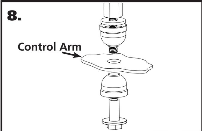
**8.** Install the End Links using **Diagram 8** as a reference. Tighten the end link barrel nut until it is flush with the end of the bolt, and then tighten it 2 more complete rounds.
