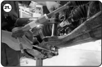
**21.** Install a 1/2" flat washer and 1/2"-13 nylok nut on the threads of each bolt sticking through the control arm. Torque the hardware to 75 ftlbs.
