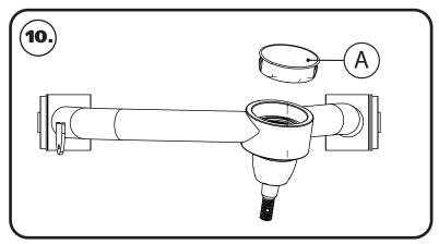
**10.** Insert the grease zerks in the ball joints. Grease the ball joints and install the supplied caps(A). These caps will help keep debris out of the control arms.
