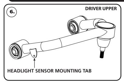
**6.** The driver upper control arm has a headlight sensor tab on the front tube. The headlight sensor is only on 2021 model year trucks. The passenger side upper control arm does NOT have this tab.
