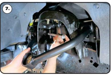
**7.** Install the Ridetech upper control arms using the OEM hardware. Again, the drivers side control arm has a headlight sensor tab on it. If installing controls arms on a 2021 F150, reattach the headlight sensor linkage to the tab of the control arm. The control arm mounting bolts will need to be tightened after the truck is sitting on the ground.
