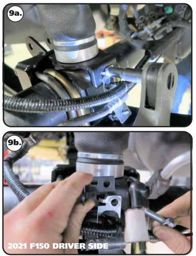
9a. & 9b. The lower mount gets attached with the M8-1.25 x 30mm & M8 flat washer supplied with the kit. 9a is 2015-2020 F150, it has no headlight sensor. 9b is 2021 F150 WITH a headlight sensor on the driver side. Align the rear tab of the lowering mount with the mounting hole in the leaf spring mount. Install the M8 flat washer on the M8-1.25 x 30 mm bolt and thread it into the OEM mounting hole. Torque to 169 in-lbs.
