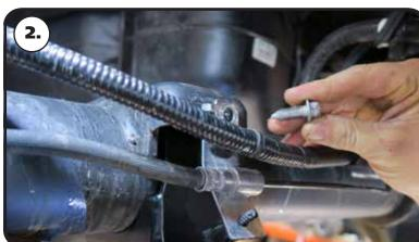
**2.** Remove the brake line bracket bolt from the rear of the leaf spring pads.
