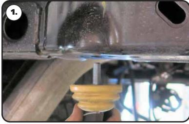
**1.** Remove the bump stops from the OEM location. It will be reinstalled to help hold the upper air spring mount in place.
