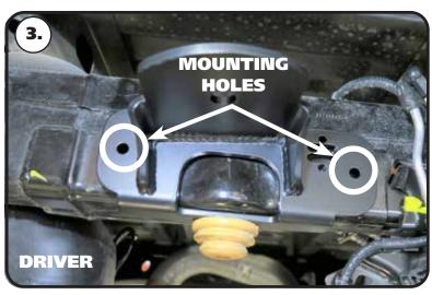
**3.** Position the upper air spring mount in place over the OEM bumpstop hole. The air spring mount is positioned with the ICON to the rear of the truck. The Driver side is shown in **Image 3.** Reinstall the bumpstop to hold the upper air spring mount in place.
