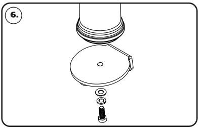
**6.** Attach the lower air spring mount to the bottom of the air spring using a 3/8"-16 x 1" bolt, 3/8" split lock washer, & 3/8" SAE flat washer. Torque to 23 ft-lbs. Repeat for the 2nd air spring & mount.
